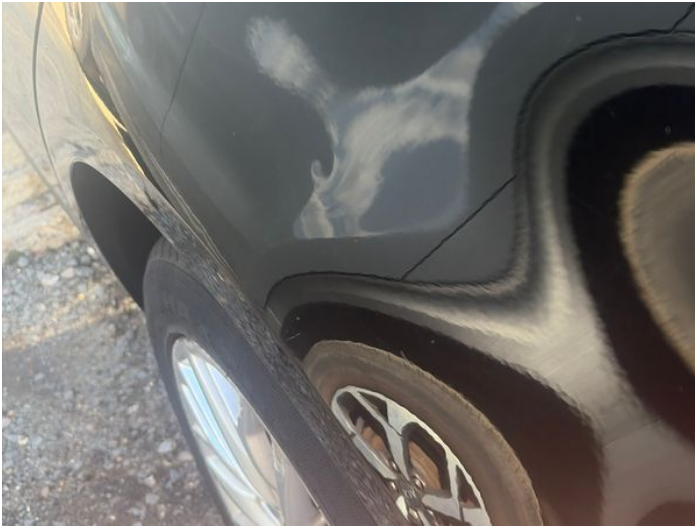
9: Qtr Panel nsr Dented Between 10mm + 30mm
