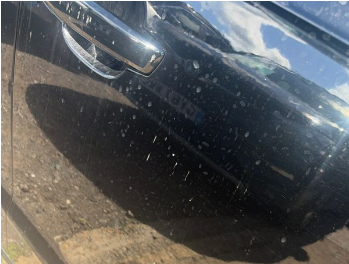
3: Door osf Chipped Multiple Chips
