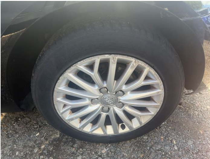
11: Wheel nsr Scratched Over 50mm
