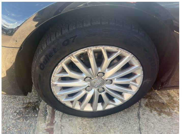
14: Wheel nsf Scratched Over 50mm
