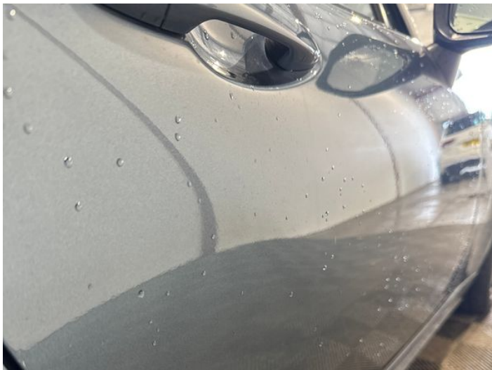
3: Door osf Poor Previous Repair Rippled UpTo 30%
