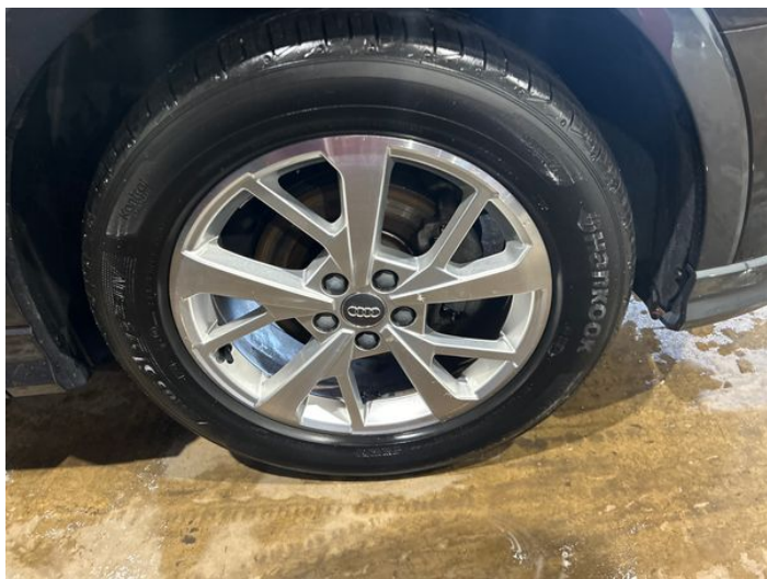
1: Wheel osf Corroded Light
