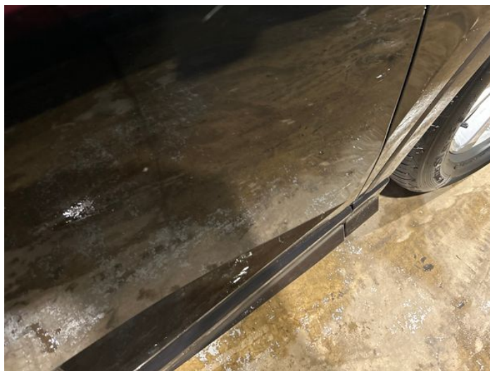
2: Door osf Scratched Over 25mm Thru Paint
