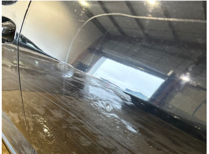
4: Door nsr Dented With Paint Damage
