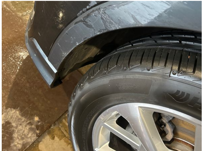
6: Wing Front Arch Extension ns Scratched (Painted) Over 25mm Thru Paint
