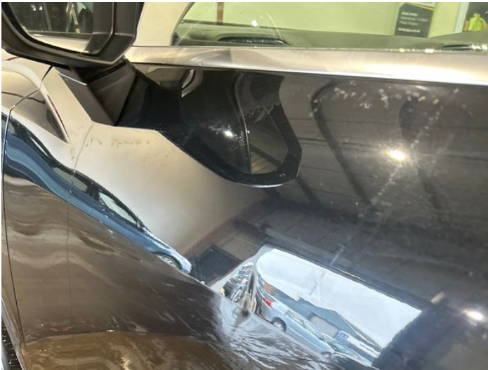
5: Door nsf Dented Over 30mm
