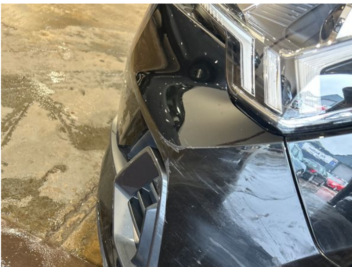
7: Bumper Front Scratched 25 to 100mm Thru Paint
