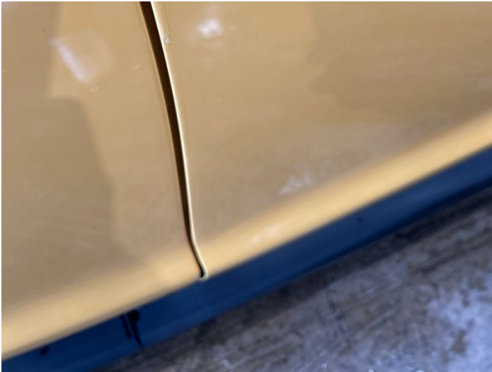
3: Door osf Poor Previous Repair Poor Paint
