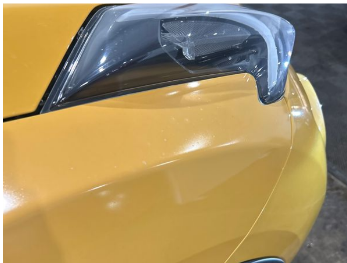
2: Wing osf Poor Previous Repair Poor Paint
