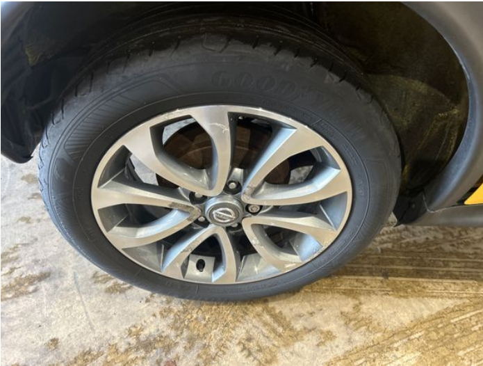
4: Wheel osr Corroded Light
