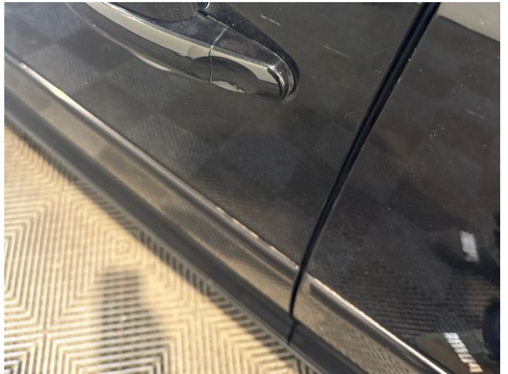
6: Door nsf Scratched UpTo 25mm Thru Paint
