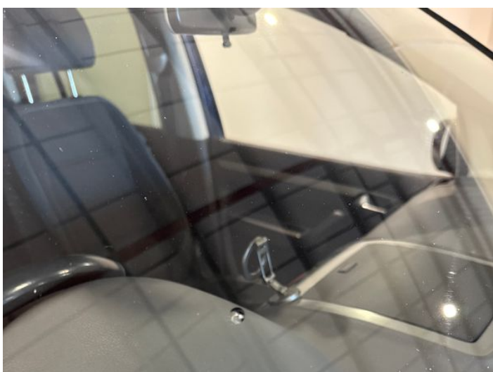
19: Screen Front Chipped UpTo 10mm
