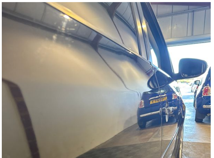
14: Door osr Dented Over 30mm
