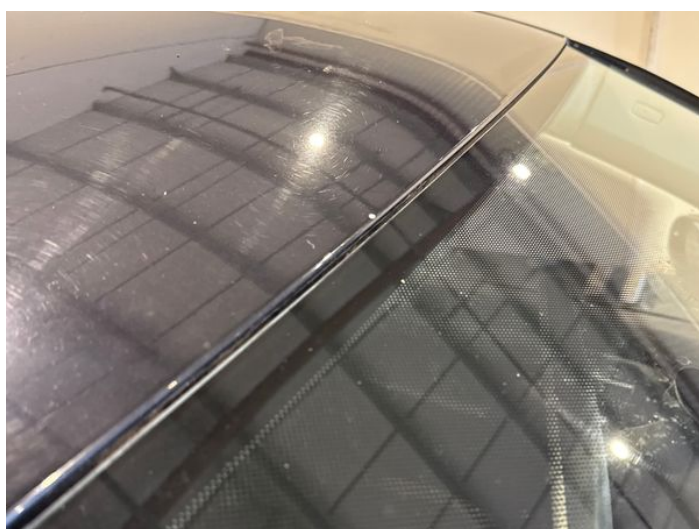
20: Roof Chipped Edge Chip
