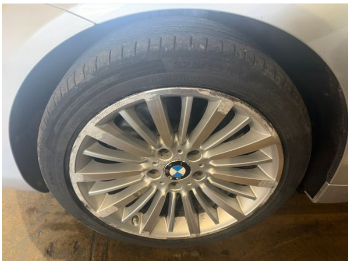
9: Wheel nsf Corroded Light
