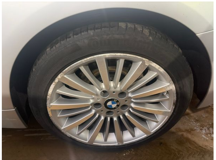
6: Wheel nsr Corroded Light
