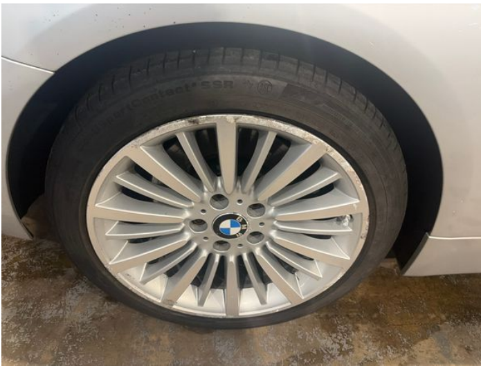
5: Wheel osr Corroded Light
