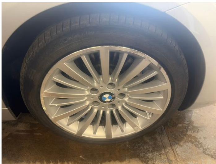
1: Wheel osf Corroded Light
