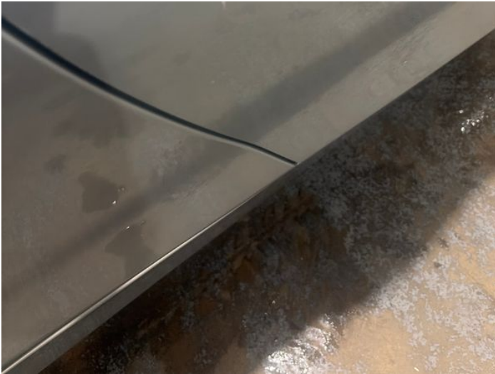
3: Door osf Scratched UpTo 25mm Thru Paint
