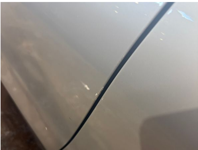
7: Door nsf Chipped Edge Chip
