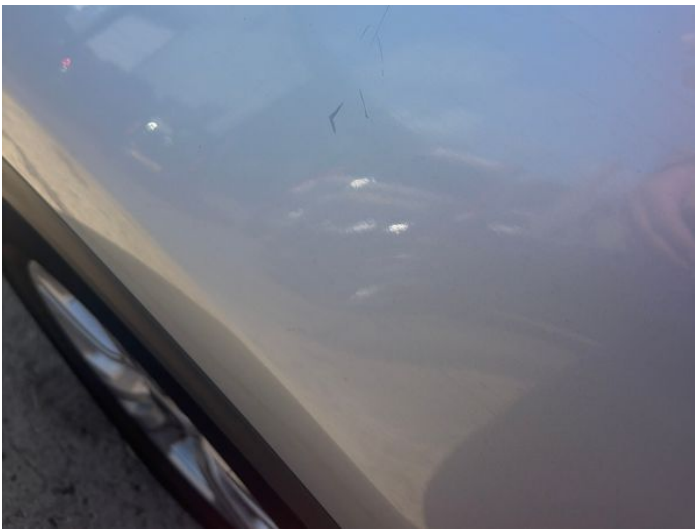
11: Wing nsf Scratched Over 25mm Thru Paint
