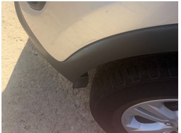
12: Bumper Front Scratched Over 100mm Thru Paint
