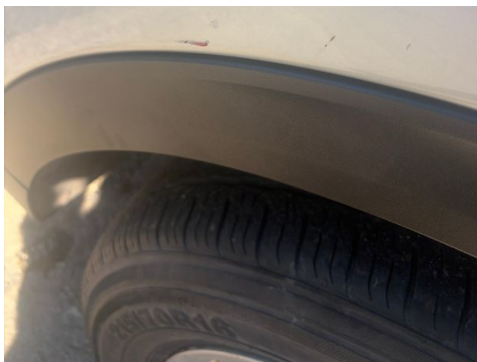
2: Wing osf Scratched UpTo 25mm Thru Paint
