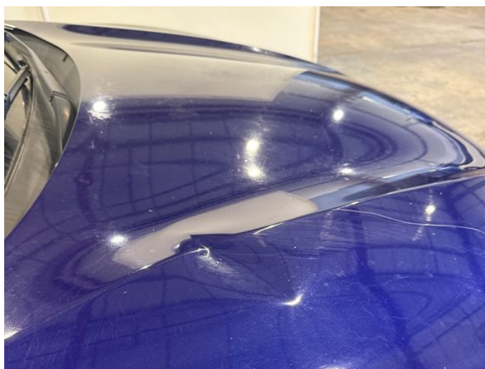
2: Bonnet Dented With Paint Damage
