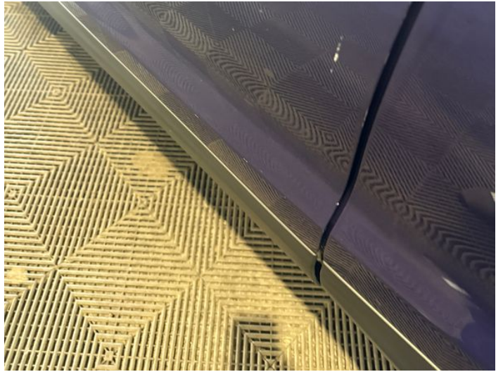
10: Door nsf Scratched Over 25mm Thru Paint
