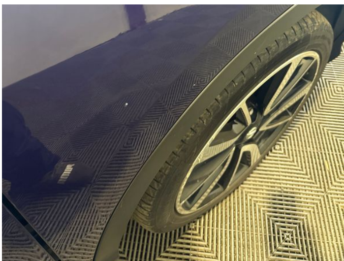
25: Wing osf Scratched UpTo 25mm Thru Paint
