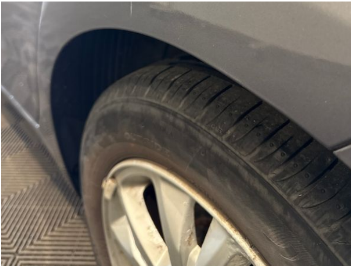
11: Qtr Panel nsr Dented Between 10mm + 30mm
