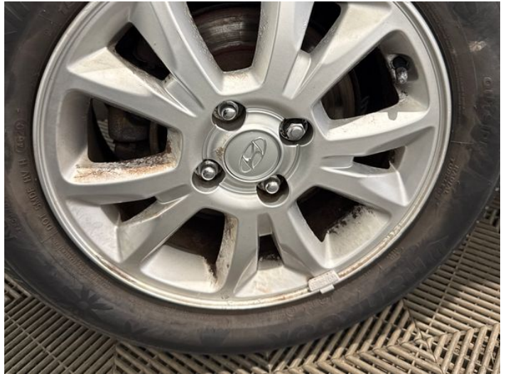
16: Wheel osr Scratched Over 50mm
