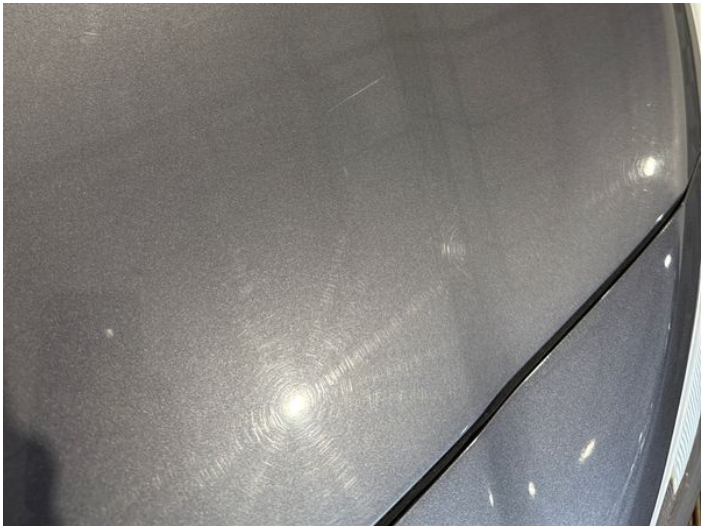
2: Bonnet Scratched Over 25mm Thru Paint
