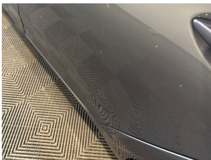
8: Door nsr Dented Between 10mm + 30mm
