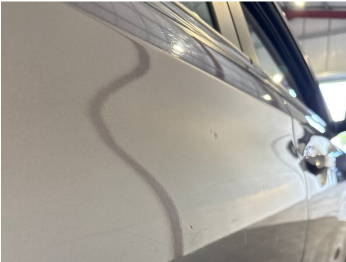
17: Door osr Dented Between 10mm + 30mm
