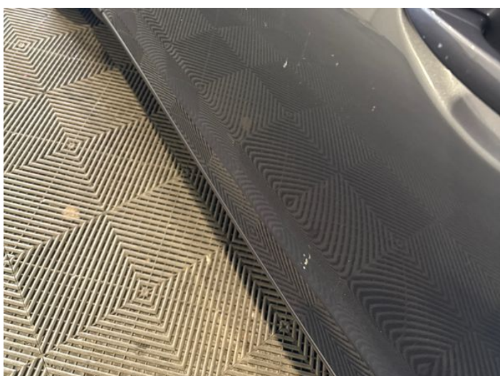
7: Door nsf Dented With Paint Damage
