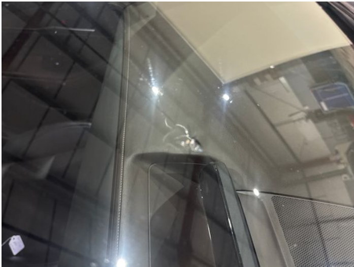
18: Screen Front Cracked Replace
