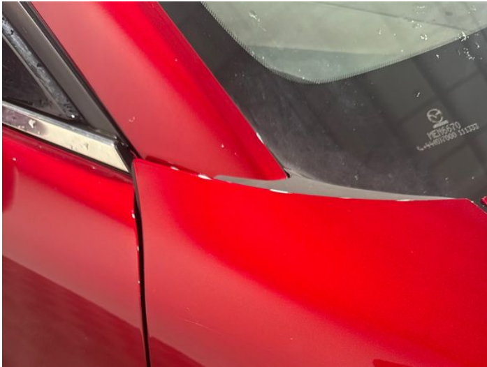
16: Wing osf Scratched UpTo 25mm Thru Paint
