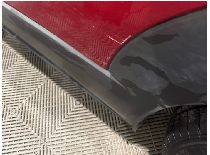
6: Door nsr Dented With Paint Damage
