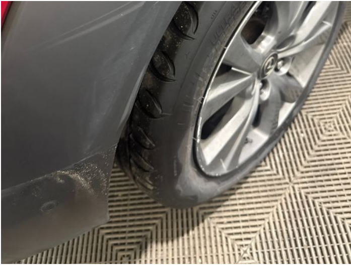
9: Qtr Panel Arch Extension os Scuffed (Unpainted) Over 100mm
