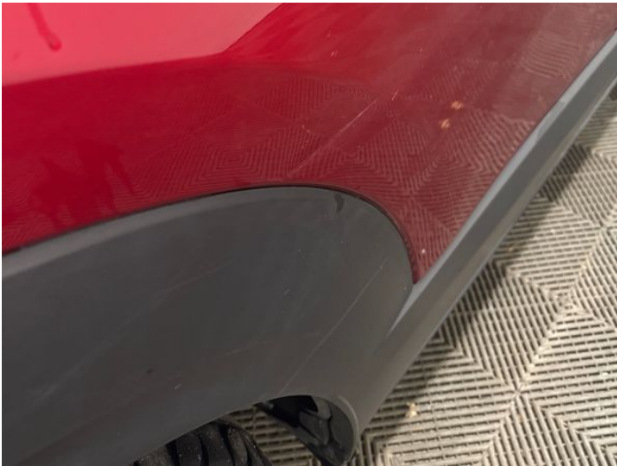
11: Door osr Scratched Over 25mm Thru Paint
