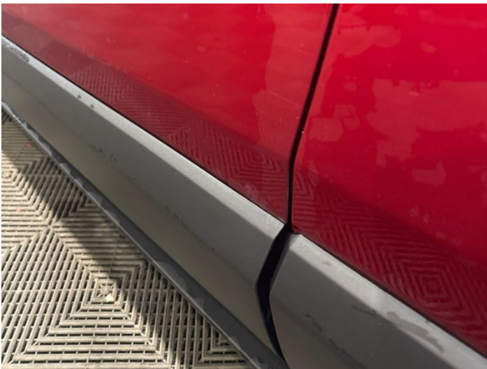
5: Door nsf Scratched UpTo 25mm Thru Paint
