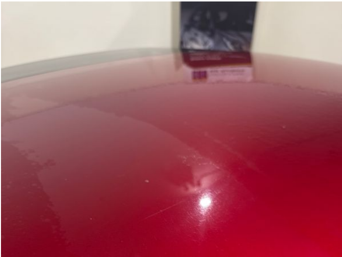
17: Roof Scratched UpTo 25mm Thru Paint
