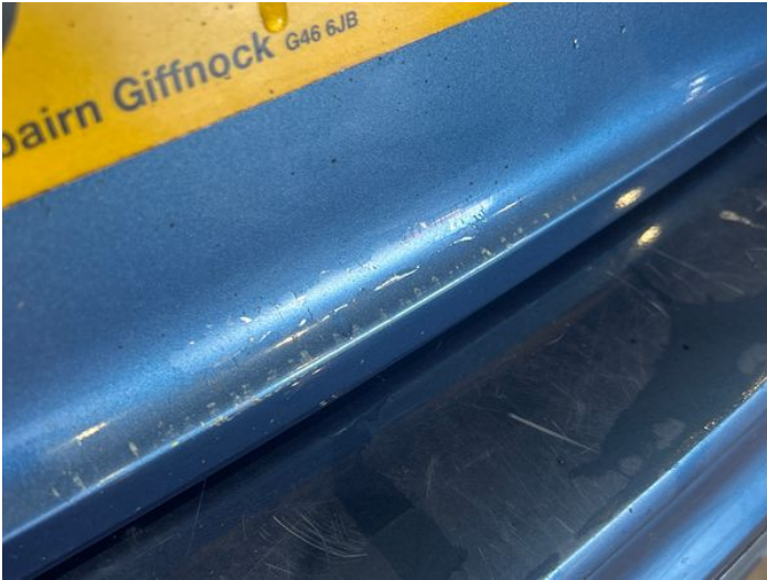
9: Tailgate Poor Previous Repair Paint Flake
