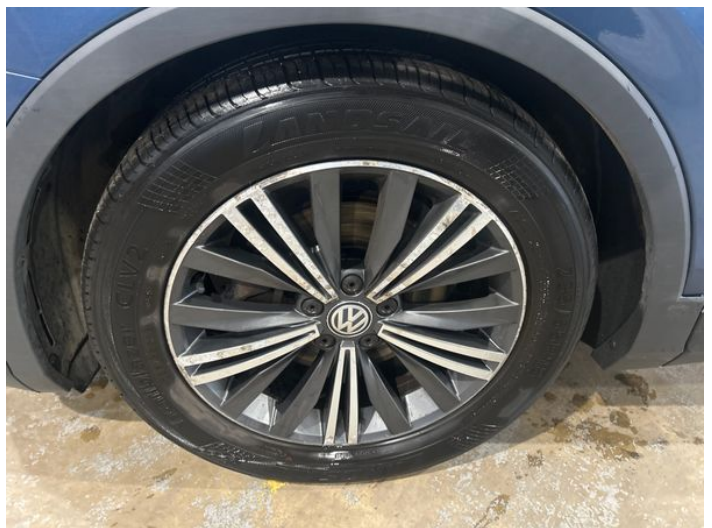
14: Wheel nsf Corroded Light
