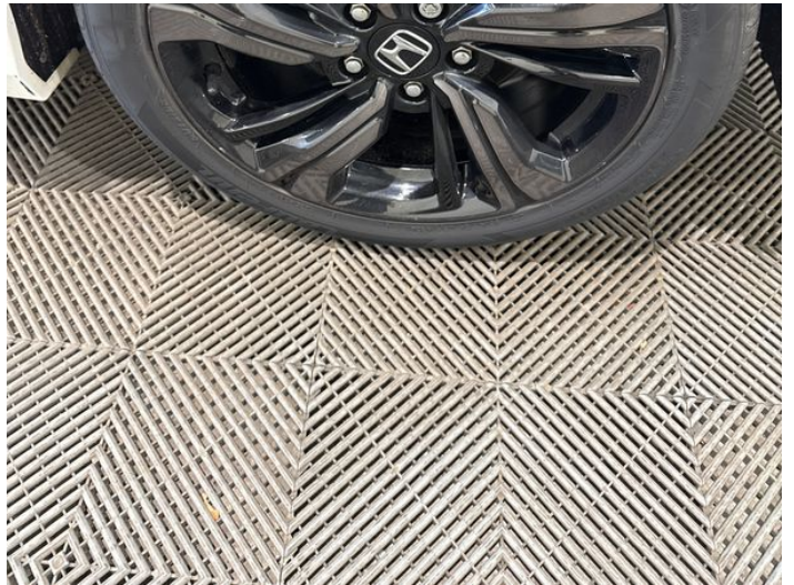
6: Wheel nsr Scratched Over 50mm
