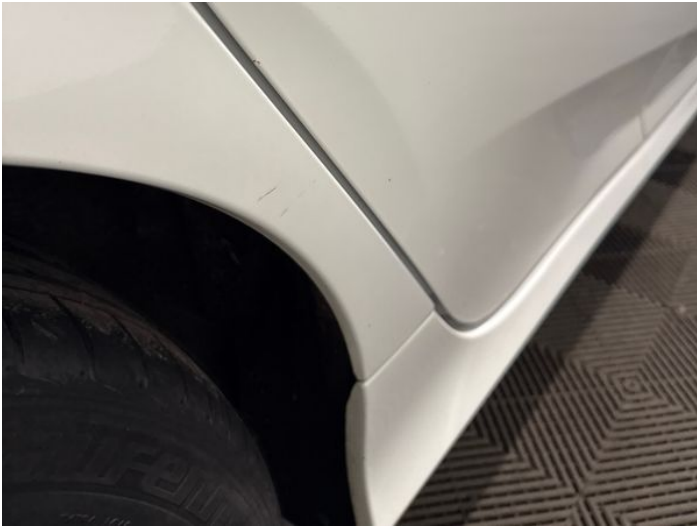
9: Door osr Chipped Edge Chip
