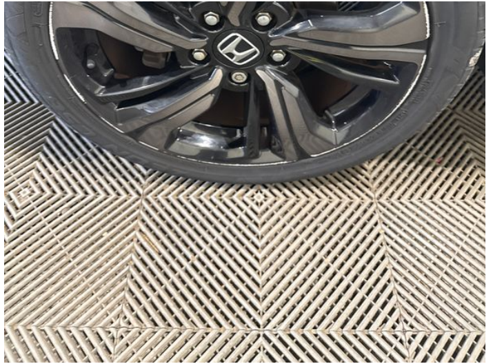
4: Wheel nsf Scratched Over 50mm
