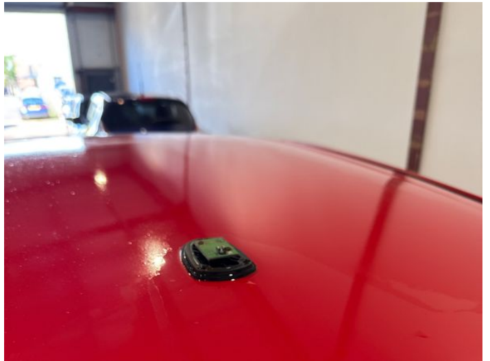
12: Aerial Broken Replace
