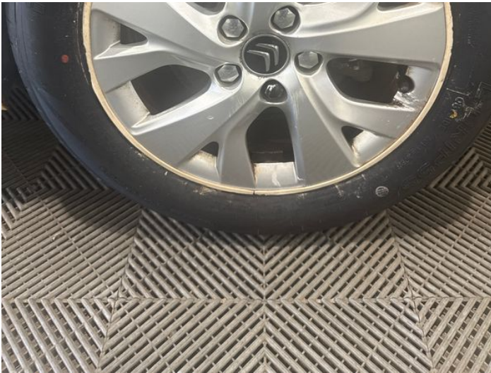
11: Wheel nsr Corroded Light
