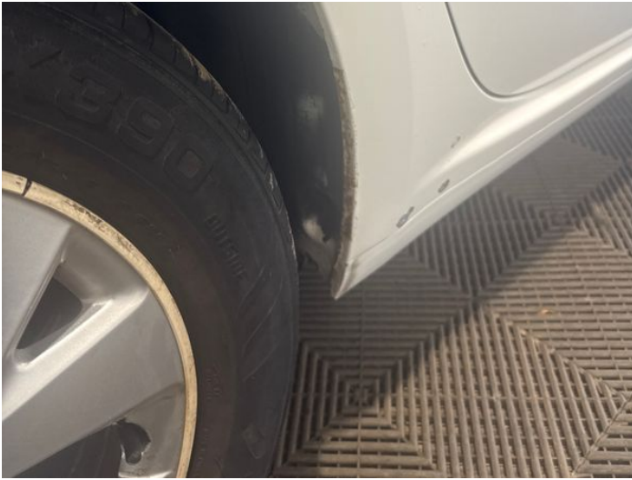
15: Qtr Panel osr Rusted Over 5mm
