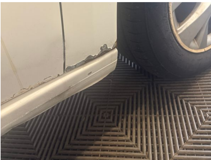
19: Wing osf Scratched Rusted
