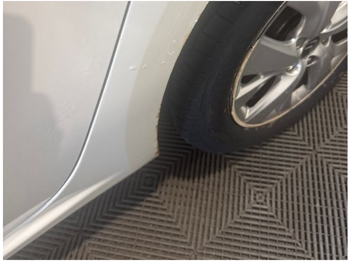
10: Qtr Panel nsr Rusted Over 5mm
