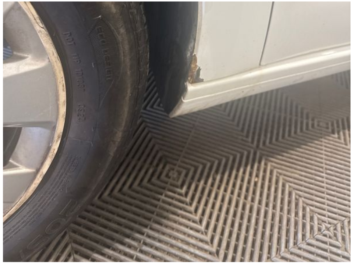
6: Wing nsf Rusted Over 5mm
