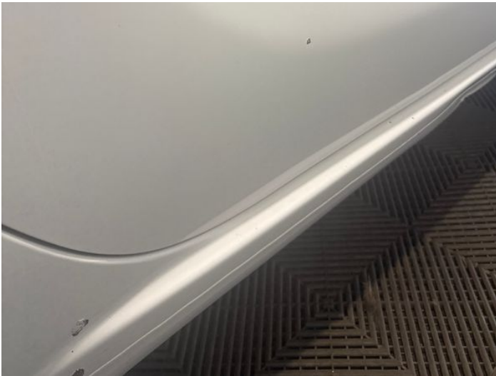
17: Door osr Chipped Over 5mm
