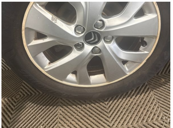
14: Wheel osr Corroded Light
