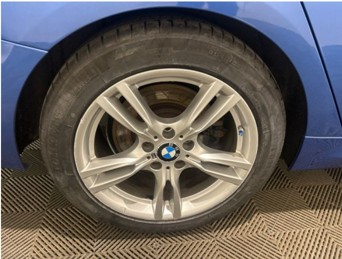
5: Wheel osr Scratched Over 50mm
