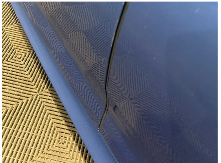
12: Door nsf Chipped Edge Chip
