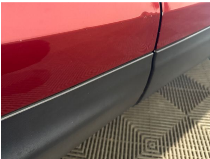
11: Door osr Dented Between 10mm + 30mm
