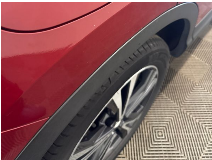
9: Qtr Panel osr Chipped 1 To 5
