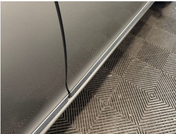
17: Door osf Chipped Edge Chip
