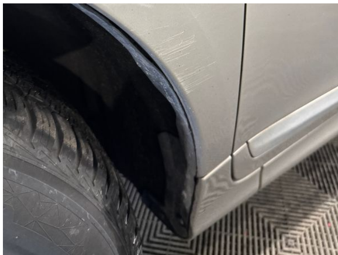
4: Wing nsf Scratched Over 25mm Thru Paint
