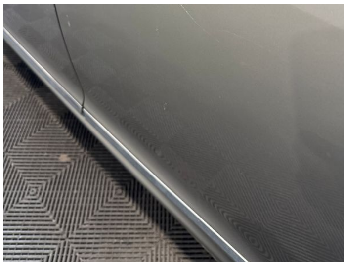
8: Door nsr Scratched Over 25mm Thru Paint
