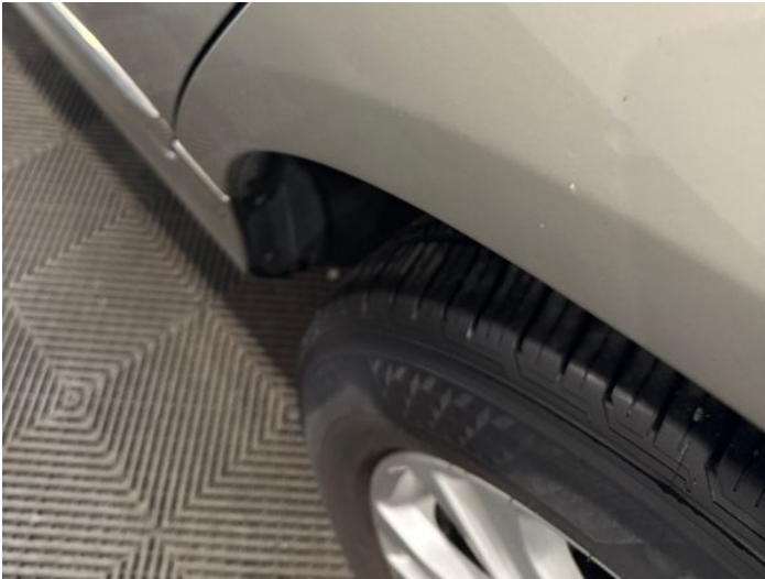
9: Qtr Panel nsr Dented Between 10mm + 30mm
