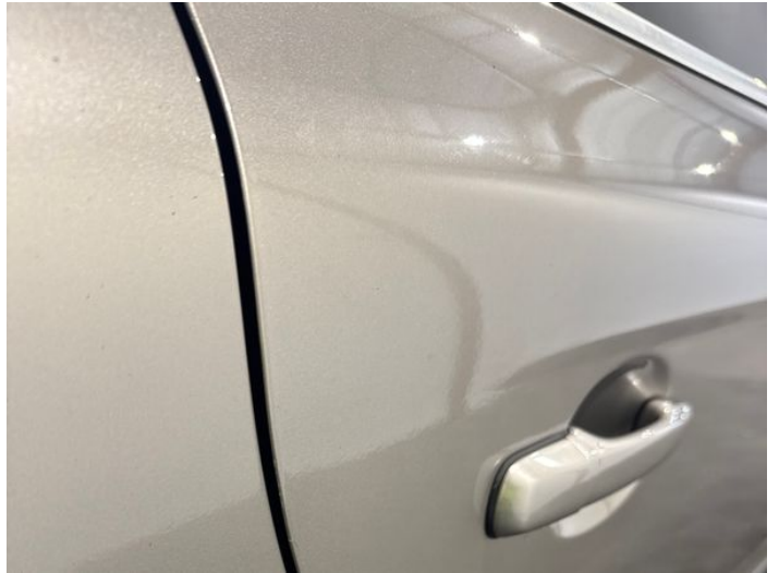
16: Door osr Poor Previous Repair Poor Paint
