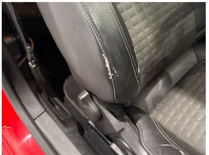
20: Seat Back Cover osf Scuffed Over 25mm
