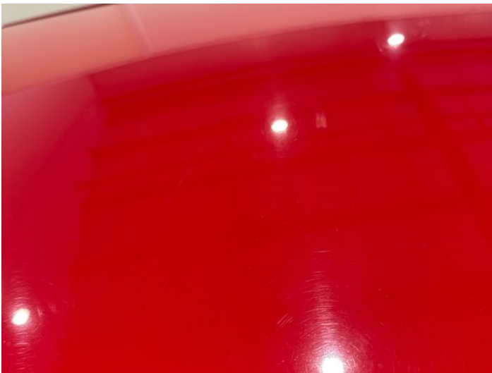
17: Roof Scratched Over 25mm Thru Paint
