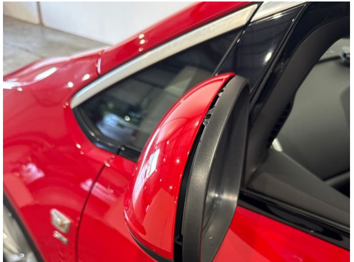
6: Door Mirror Assy nsf Broken Replace
