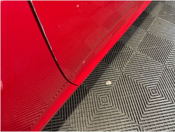
15: Door osf Scratched Over 25mm Thru Paint
