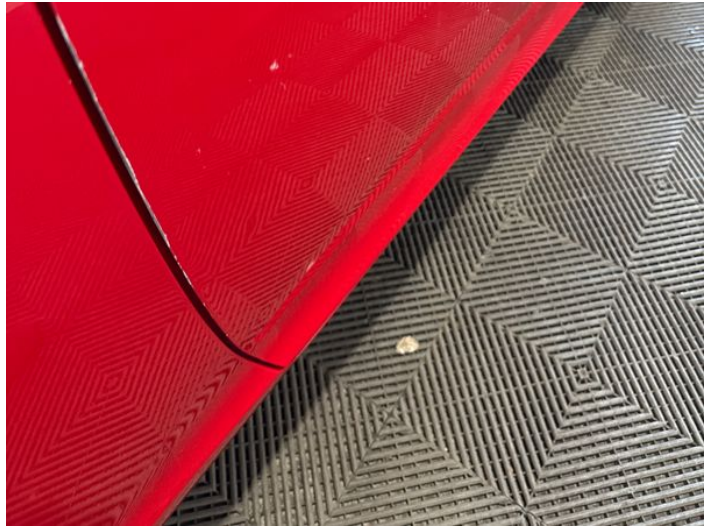
16: Door osf Dented Between 10mm + 30mm
