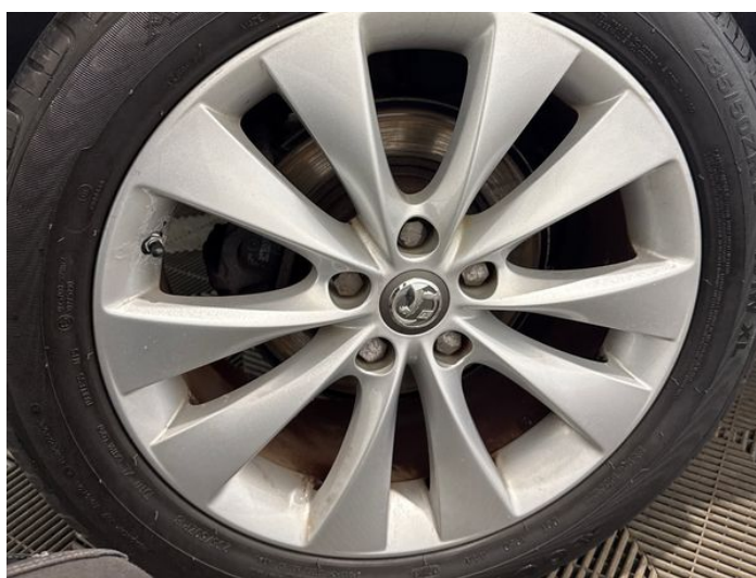
14: Wheel osr Corroded Light
