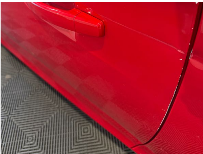
7: Door nsf Dented With Paint Damage
