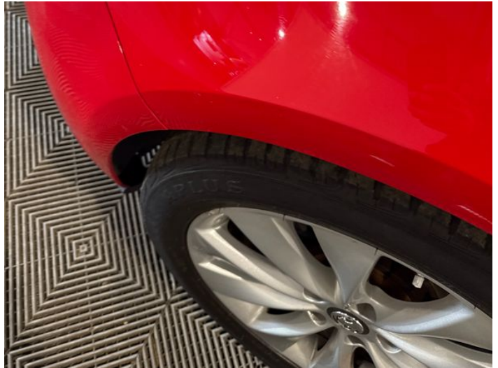
4: Wing nsf Chipped Multiple Chips
