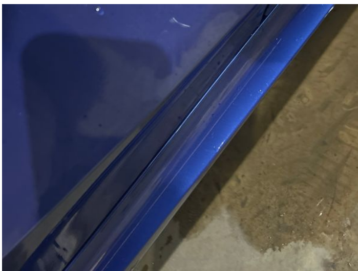
5: Door osr Scratched UpTo 25mm Thru Paint
