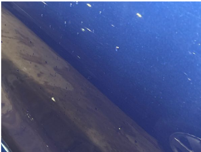
3: Door osf Chipped 1 To 5
