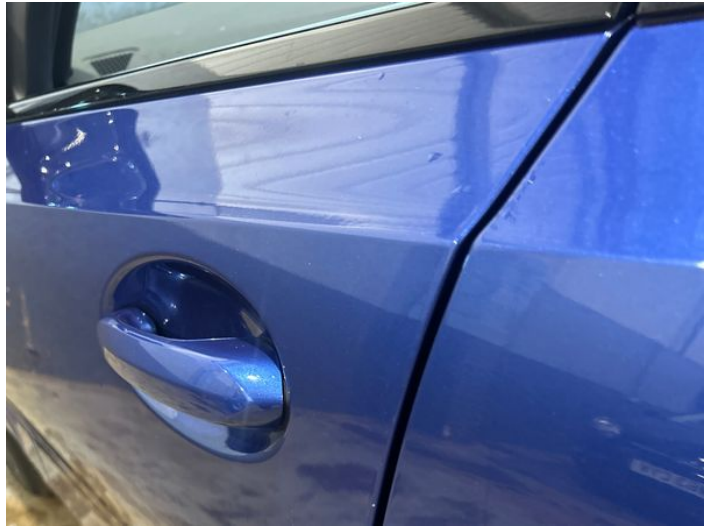
10: Door nsf Chipped Edge Chip
