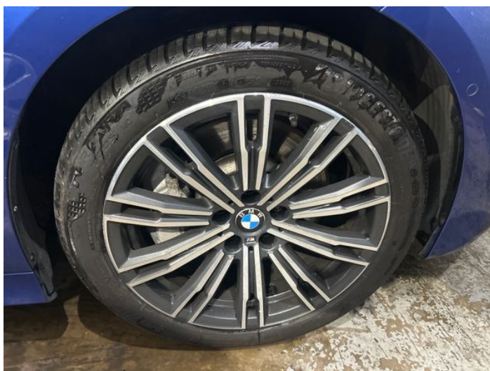
1: Wheel osf Corroded Light
