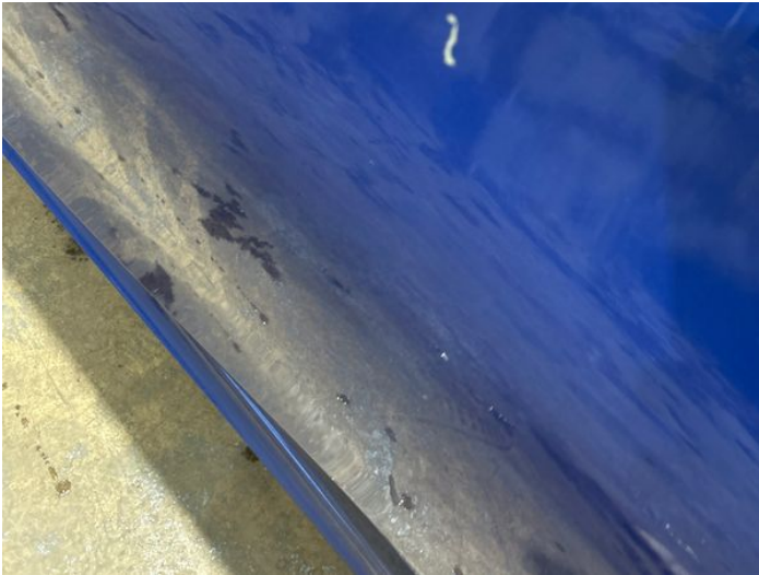
9: Door nsr Scratched UpTo 25mm Thru Paint
