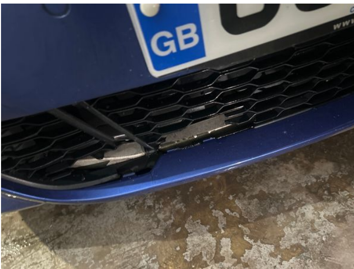
13: Bumper Front Grill Broken Replace
