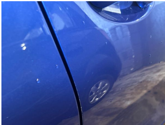
4: Door osf Chipped Edge Chip
