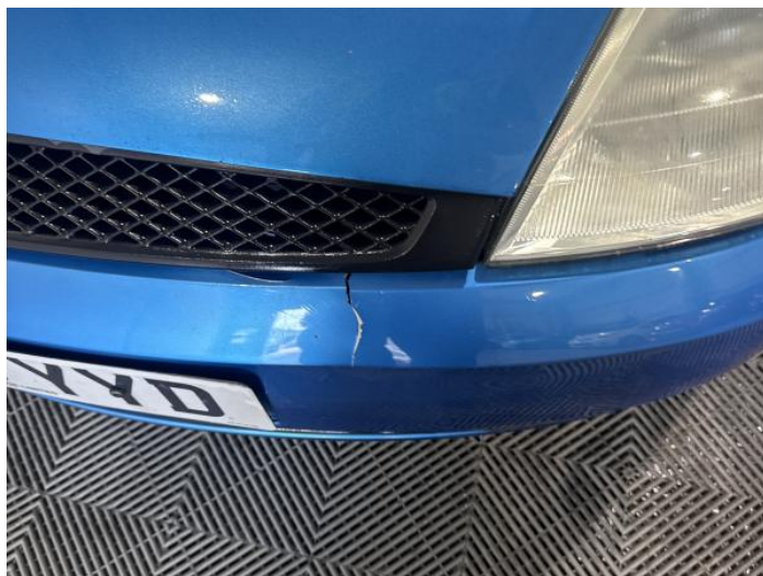
2: Bumper Front Cracked Over 25mm
