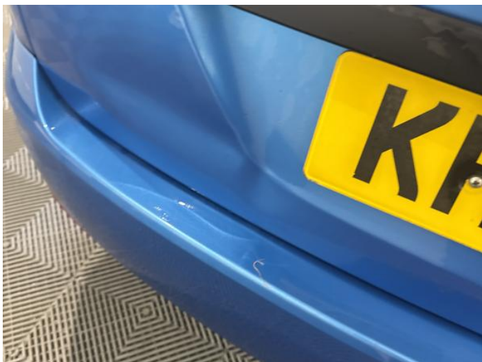
9: Boot Lid Dented Over 30mm
