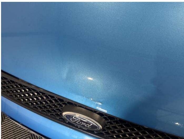
1: Bonnet Dented With Paint Damage
