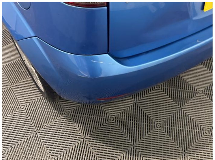
8: Bumper Rear Poor Previous Repair Rippled Up To 30%
