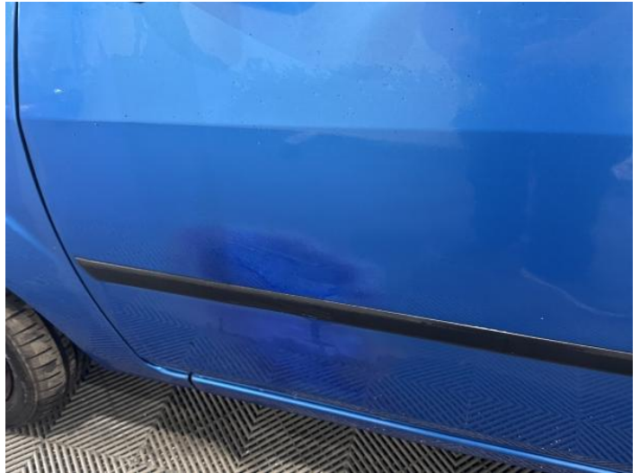
4: Door nsf Poor Previous Repair Poor Paint
