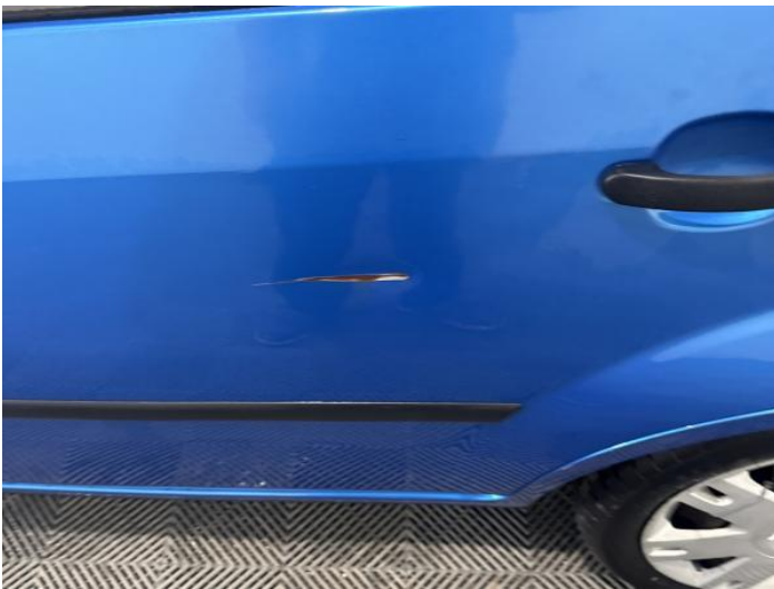
5: Door nsr Dented With Paint Damage
