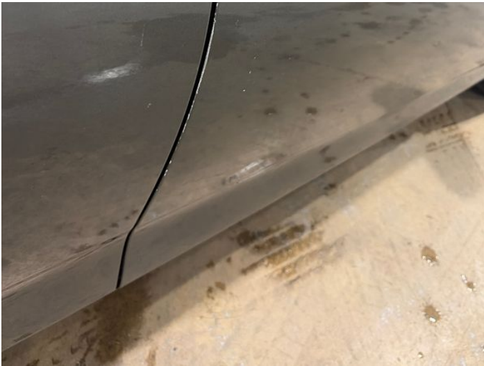
5: Door osf Chipped Edge Chip
