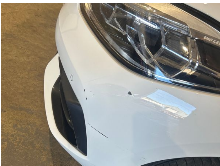
5: Bumper Front Scratched 25 to 100mm Thru Paint
