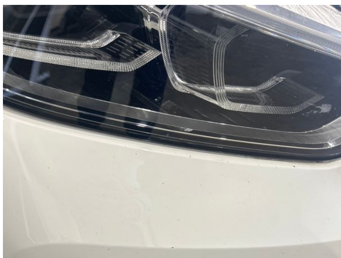
6: Bumper Front Chipped Multiple Chips
