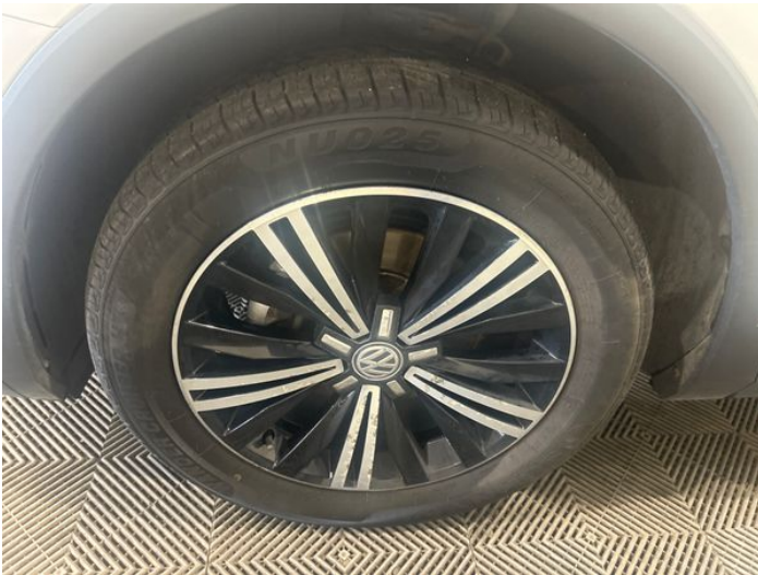
11: Wheel nsf Corroded Light
