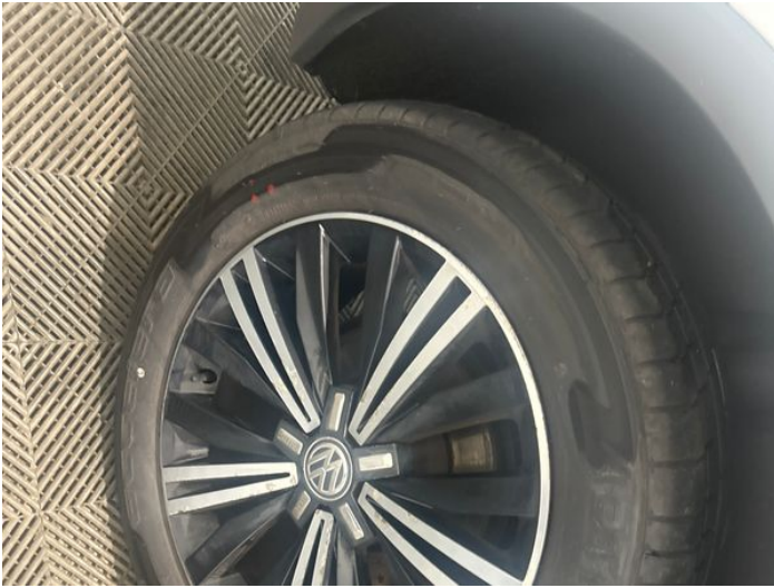
3: Wheel osr Corroded Light
