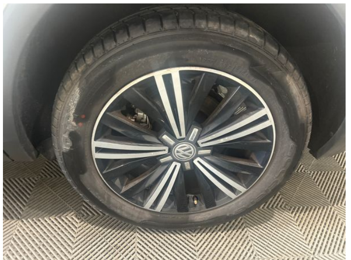
8: Wheel nsr Corroded Light
