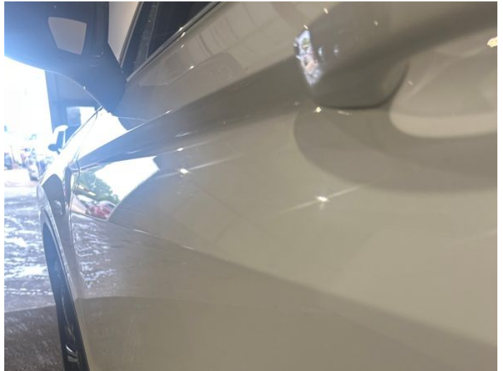
10: Door nsf Dented Between 10mm + 30mm
