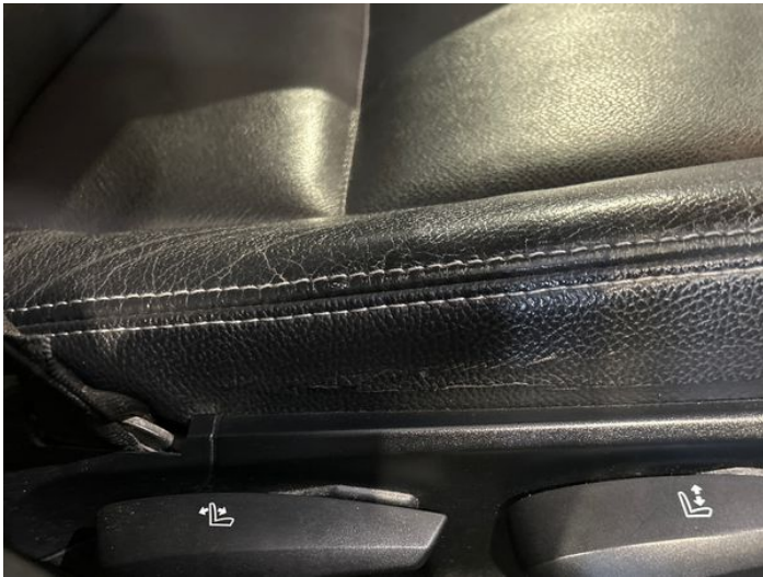
12: Seat Base Cover osf Torn Over 3mm
