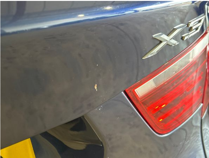
5: Tailgate Chipped 1 To 5
