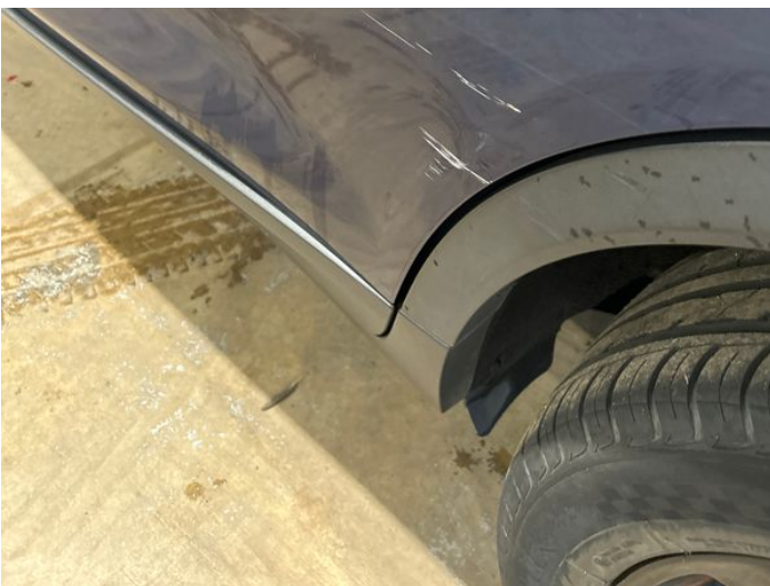
7: Door nsr Scratched Over 25mm Thru Paint
