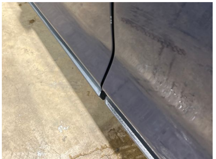
8: Door nsf Chipped Edge Chip
