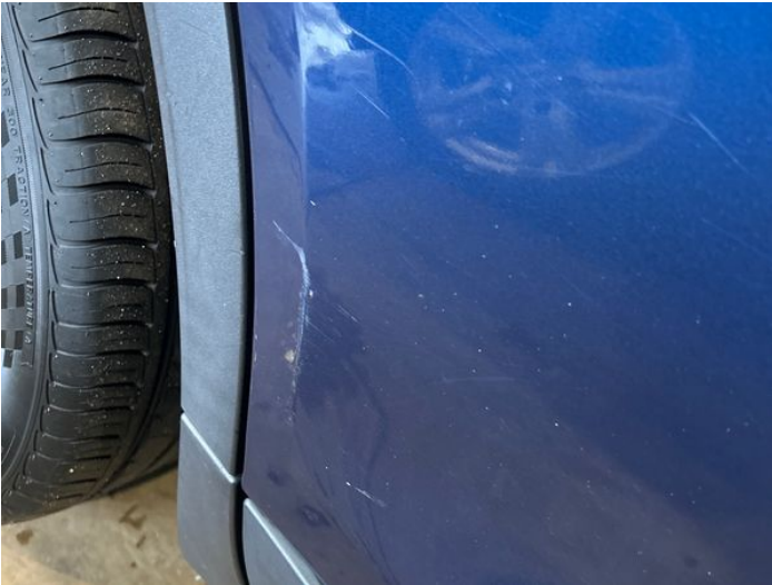
3: Door osr Scratched Over 25mm Thru Paint
