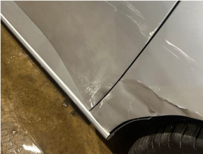
3: Door osf Dented With Paint Damage
