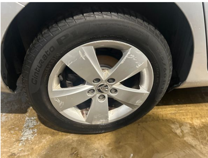
7: Wheel osr Scratched Over 50mm
