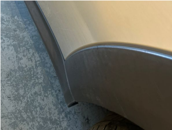
9: Qtr Panel nsr Dented Over 30mm
