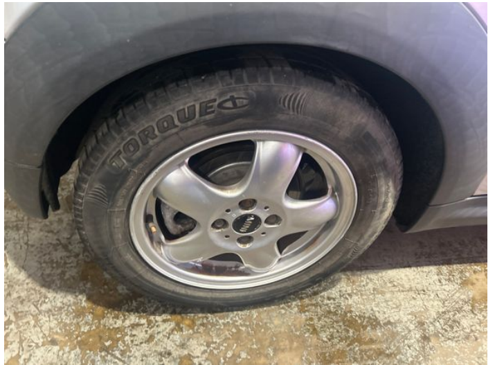
6: Wheel osr Scratched Over 50mm
