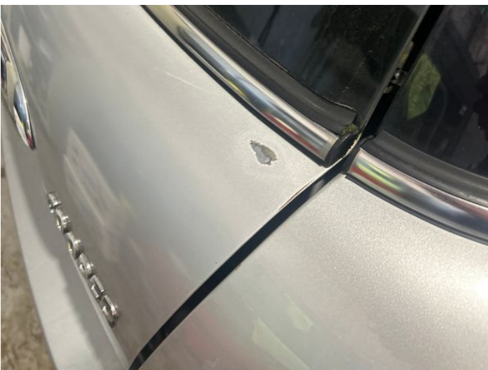
7: Tailgate Poor Previous Repair Poor Paint
