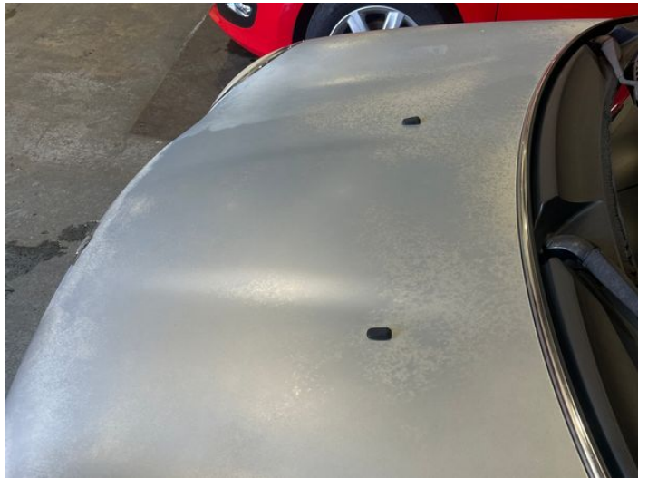
12: Bonnet Poor Previous Repair Paint Flake
