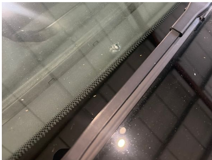
16: Screen Front Chipped UpTo 10mm
