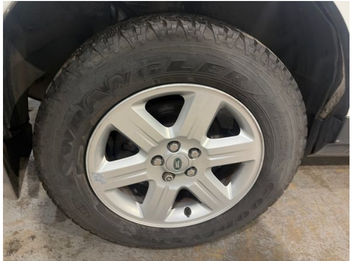
4: Wheel osr Corroded Light
