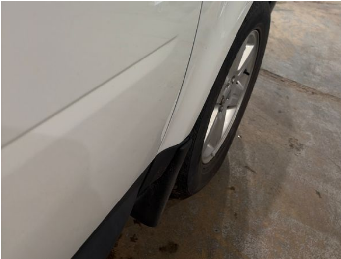
5: Door osf Dented Between 10mm + 30mm
