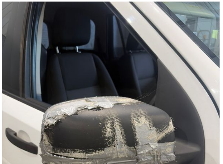
2: Door Mirror Assy osf Broken Replace
