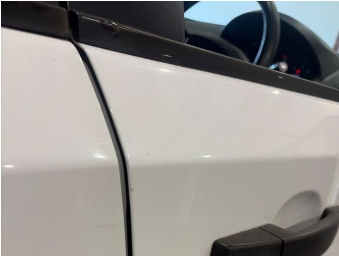
3: Door osf Chipped Edge Chip
