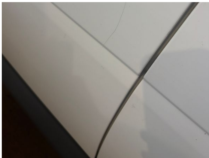
10: Door nsf Scratched Over 25mm Thru Paint
