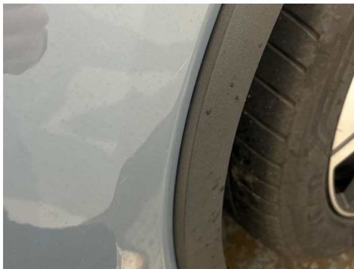
2: Wing osf Scratched UpTo 25mm Thru Paint
