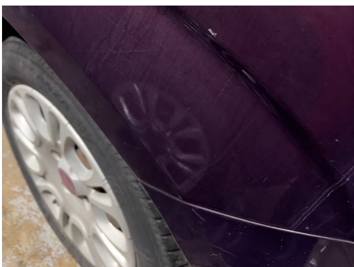
7: Qtr Panel nsr Chipped 1 To 5
