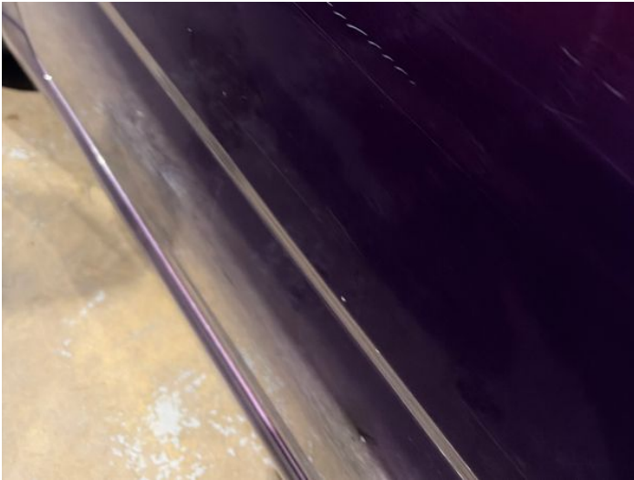
9: Door nsf Scratched Over 25mm Thru Paint
