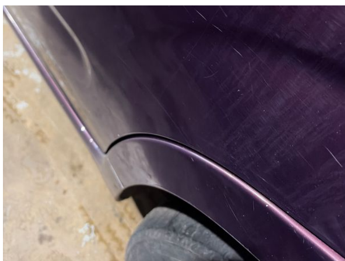
8: Door nsr Dented With Paint Damage
