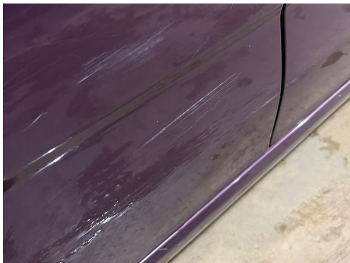
4: Door osr Scratched Over 25mm Thru Paint
