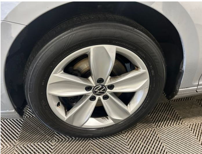
5: Wheel nsf Scratched Up To 50mm
