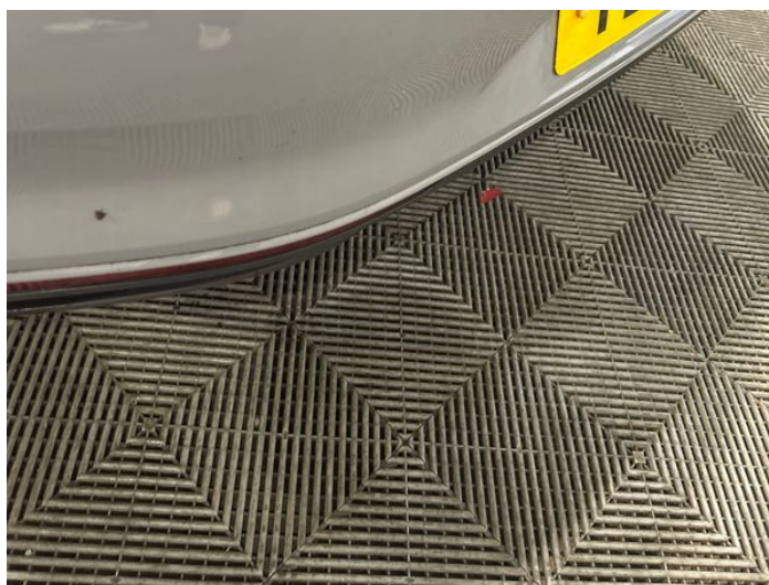
2: Bumper Rear Chipped Multiple Chips
