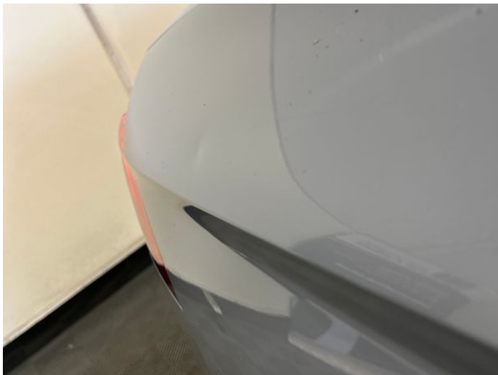
9: Qtr Panel osr Dented Between 10mm + 30mm
