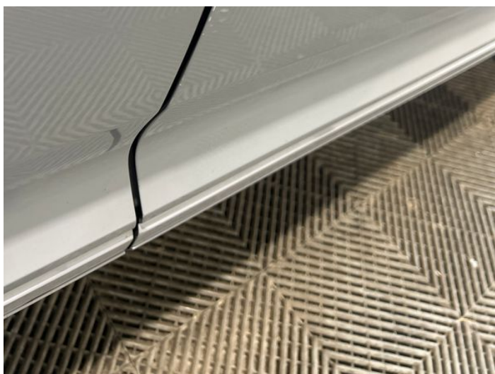
1: Door osf Chipped Edge Chip
