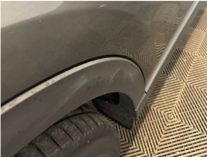
11: Door osr Scratched Over 25mm Thru Paint
