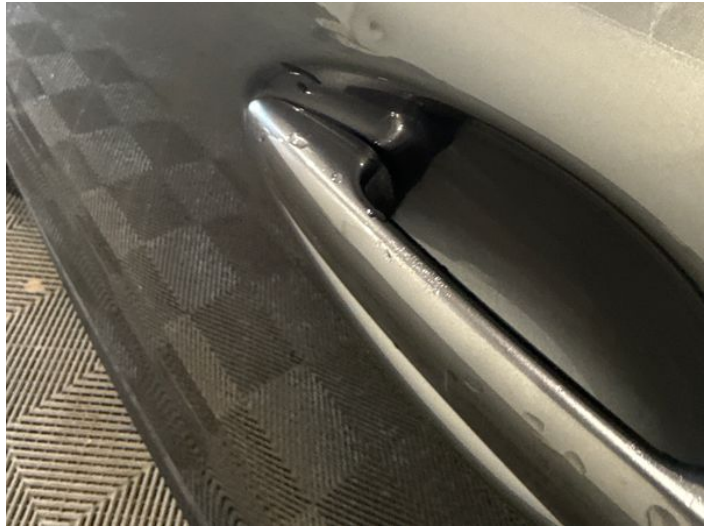
4: Door nsf Dented Between 10mm + 30mm
