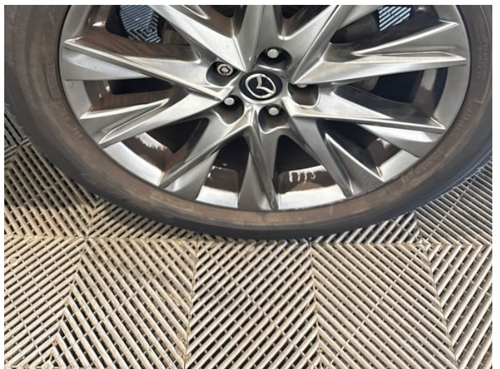
14: Wheel osf Scratched Up To 50mm
