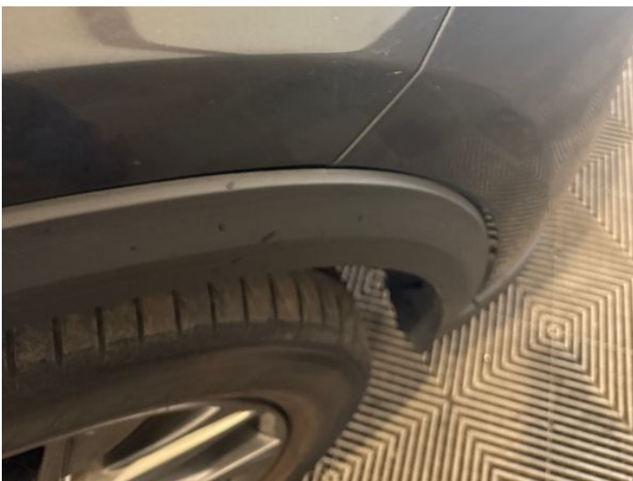
13: Wing osf Scratched UpTo 25mm Thru Paint
