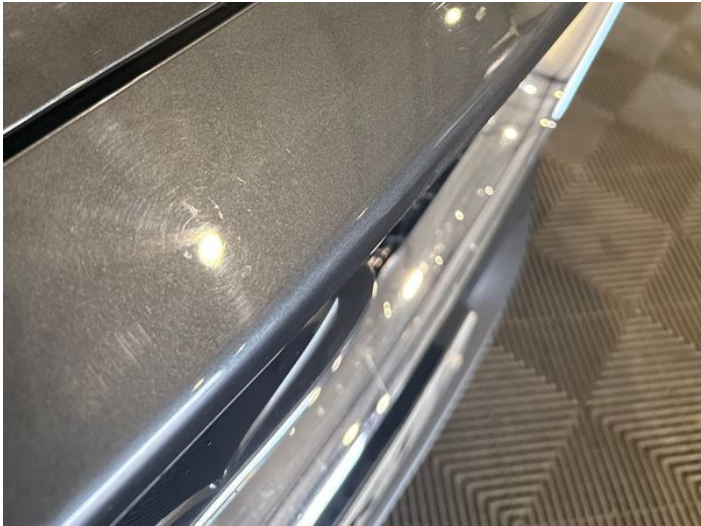
16: Bumper Front Dented With Paint Damage
