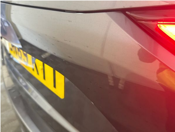
15: Tailgate Trim Panel Scratched (Painted) Over 25mm Thru Paint
