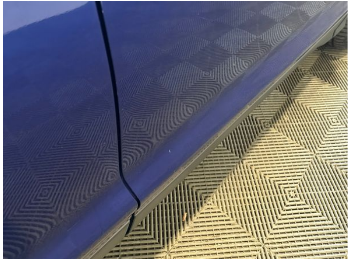
16: Door osf Chipped Edge Chip
