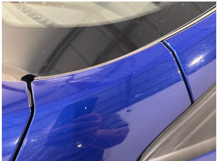
4: Wing nsf Scratched Over 25mm Thru Paint
