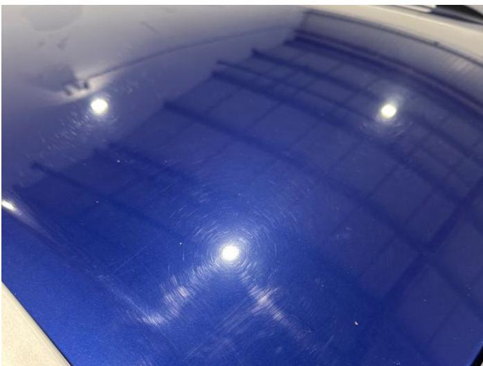
19: Roof Scratched Over 25mm Thru Paint
