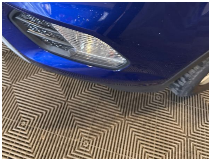
2: Bumper Front Scratched 25 to 100mm Thru Paint
