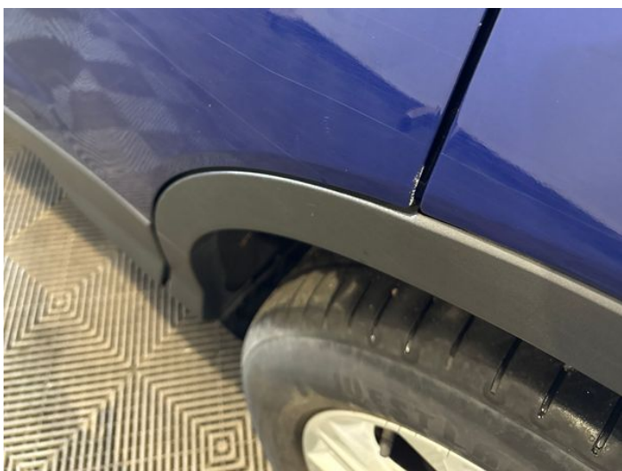
7: Door nsr Scratched Over 25mm Thru Paint
