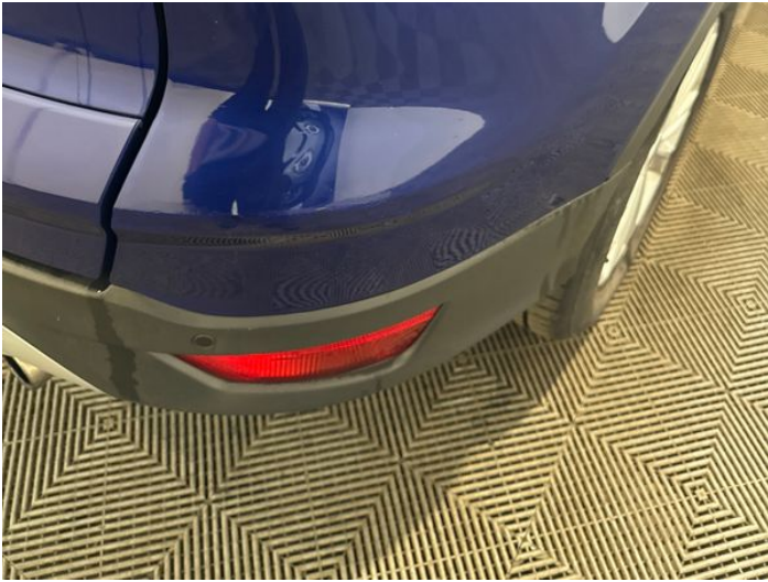
9: Bumper Rear Scratched 25 to 100mm Thru Paint
