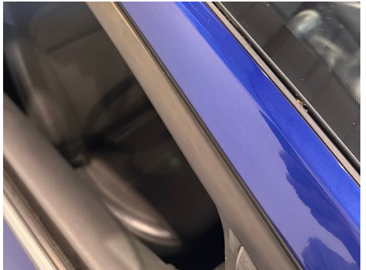
18: A Post os Scratched Over 25mm Thru Paint
