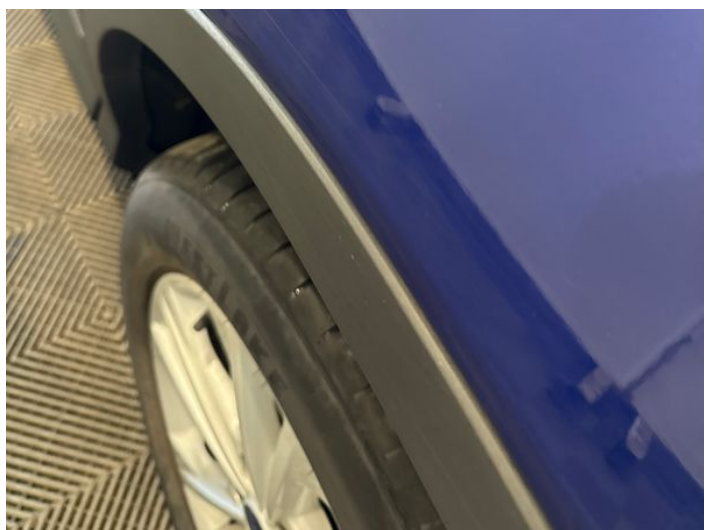
8: Qtr Panel nsr Dented Between 10mm + 30mm
