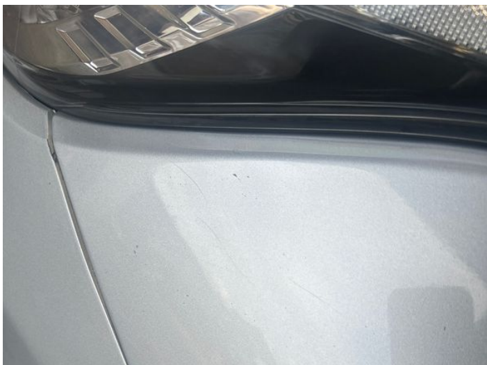
9: Wing nsf Chipped Multiple Chips
