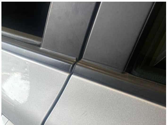
8: Door nsr Scratched UpTo 25mm Thru Paint
