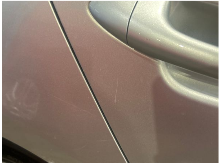
4: Door osr Scratched UpTo 25mm Thru Paint
