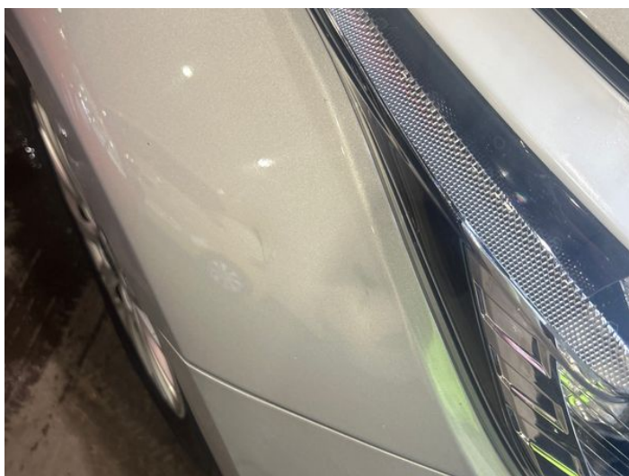
1: Wing osf Dented Over 30mm
