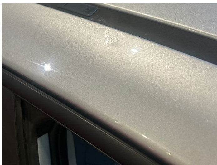
14: B Post os Dented With Paint Damage
