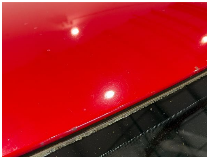
24: Roof Chipped Edge Chip
