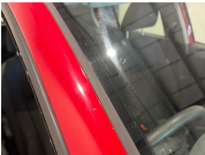
23: A Post os Chipped 1 To 5
