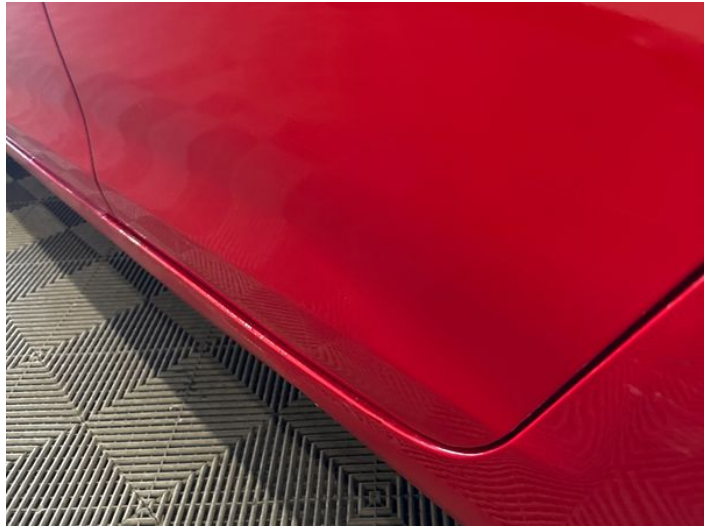
10: Door nsr Poor Previous Repair Poor Paint
