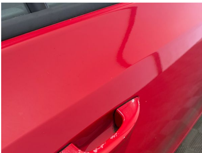
19: Door osr Scratched Over 25mm Thru Paint
