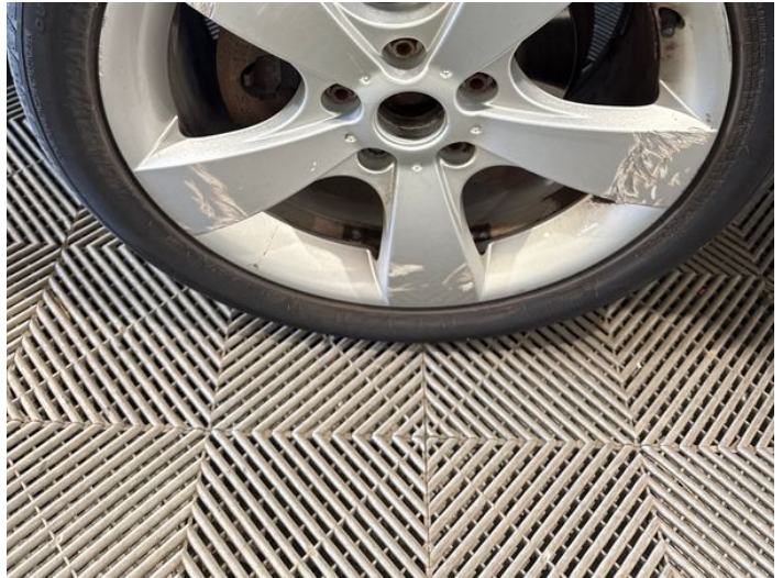
4: Wheel nsf Scratched Over 50mm
