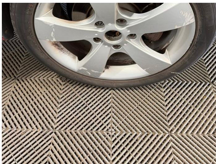
26: Wheel osf Scratched Over 50mm
