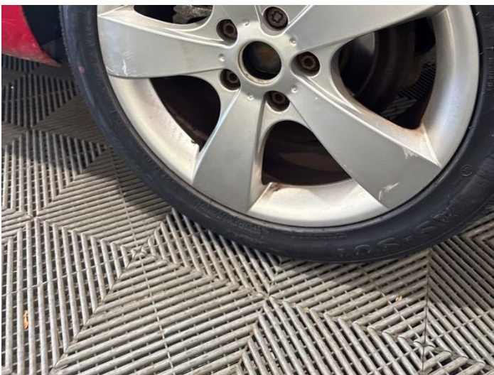
13: Wheel nsr Scratched Over 50mm
