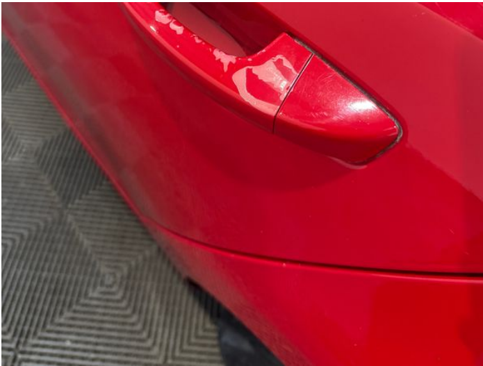
11: Door nsr Scratched Over 25mm Thru Paint
