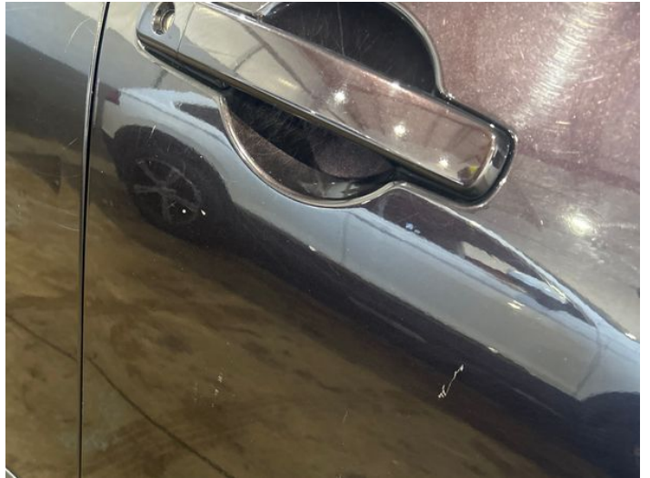
4: Door osf Chipped Multiple Chips
