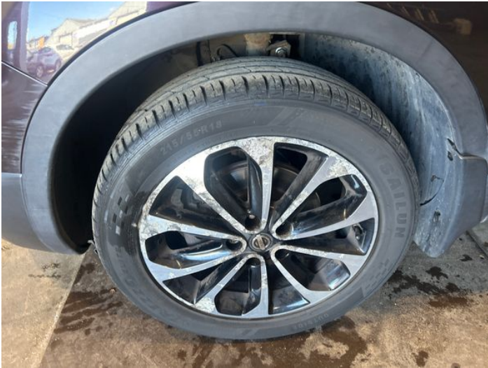
15: Wheel nsf Corroded Light
