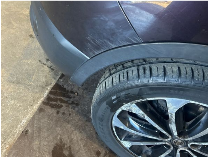
16: Bumper Front Scratched Over 100mm Thru Paint
