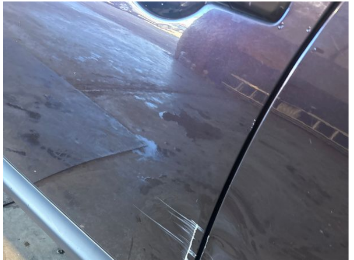
12: Door nsf Dented With Paint Damage
