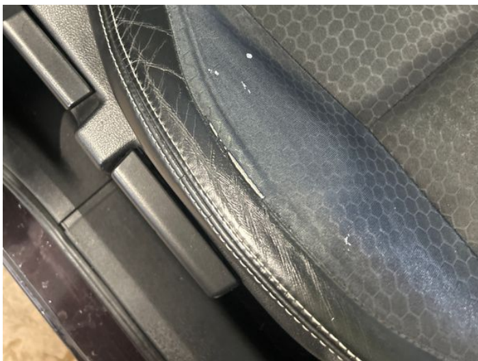
1: Seat Base Cover osf Torn Over 3mm
