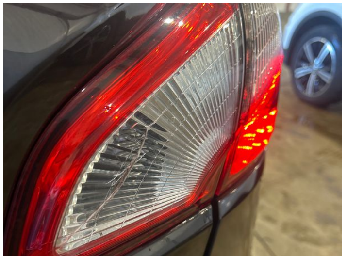
8: Lamp osr Broken Replace
