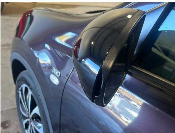
13: Door Mirror Assy nsf Broken Replace
