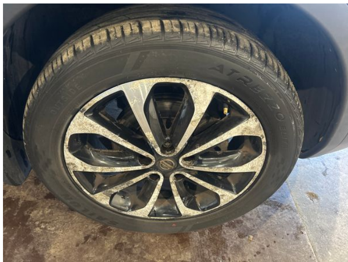
2: Wheel osf Corroded Light
