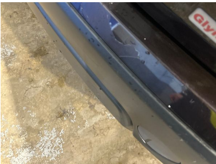
7: Bumper Rear Poor Previous Repair Paint Flake
