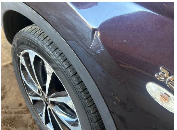
14: Wing nsf Dented With Paint Damage
