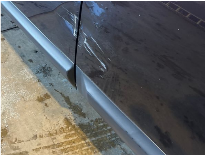
11: Door nsr Dented With Paint Damage
