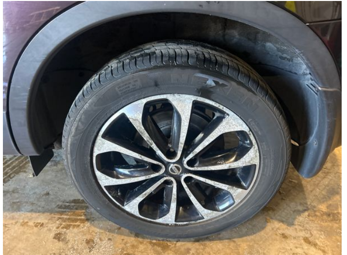
10: Wheel nsr Corroded Light
