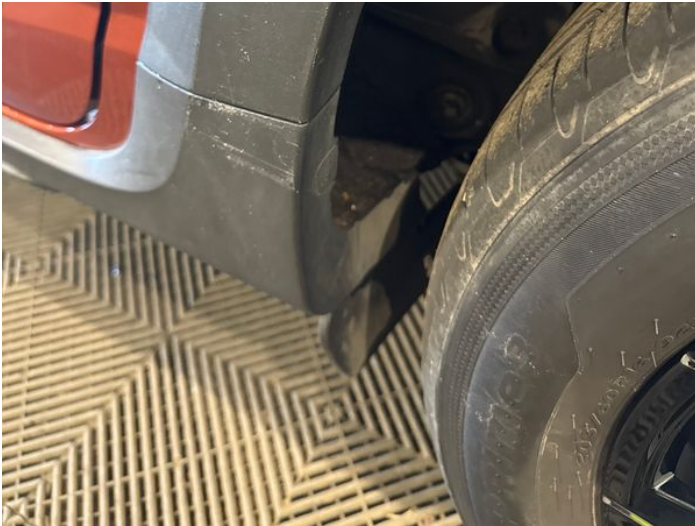
9: Qtr Panel Arch Extension ns Scuffed (Unpainted) UpTo 100mm
