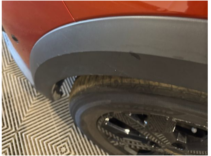
4: Wing nsf Scratched Over 25mm Thru Paint
