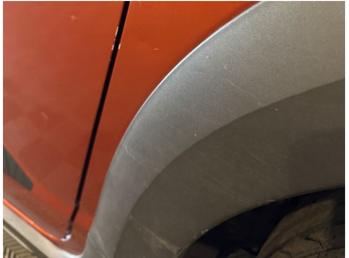
10: Qtr Panel nsr Dented Between 10mm + 30mm
