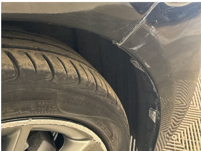
21: Wing osf Scratched UpTo 25mm Thru Paint
