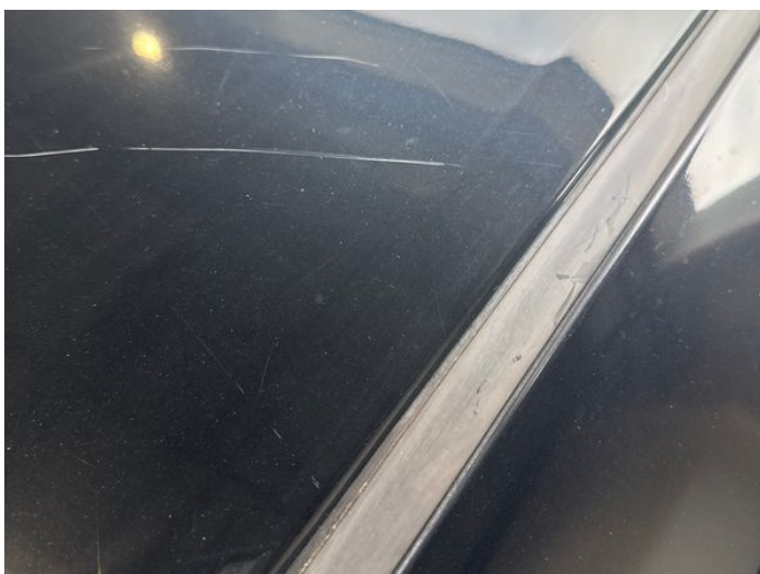
26: Roof Scratched Over 25mm Thru Paint
