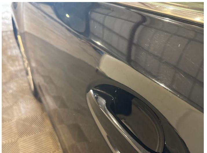
8: Door nsf Dented Over 30mm
