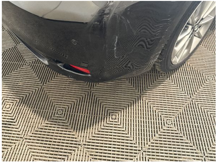
12: Bumper Rear Scratched Over 100mm Thru Paint
