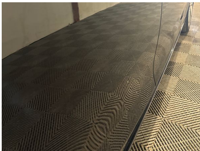
18: Door osr Dented Between 10mm + 30mm
