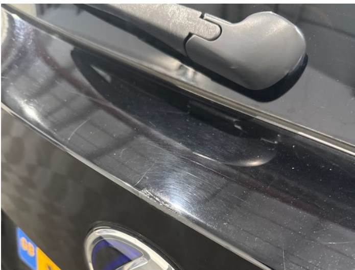
13: Tailgate Scratched Over 25mm Thru Paint
