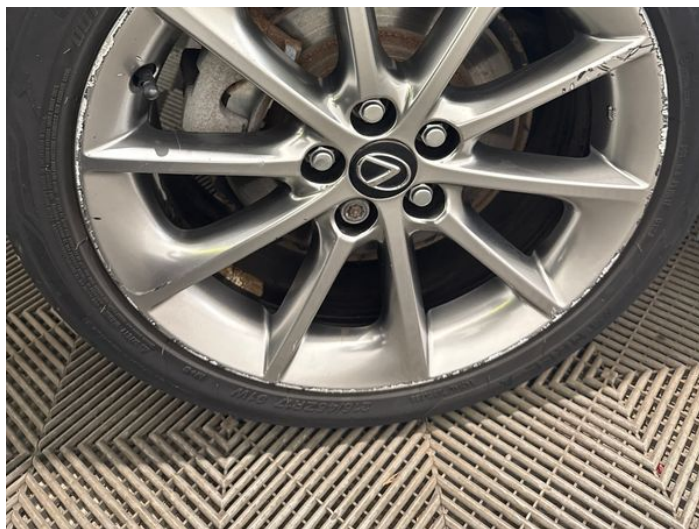
16: Wheel osr Scratched Over 50mm
