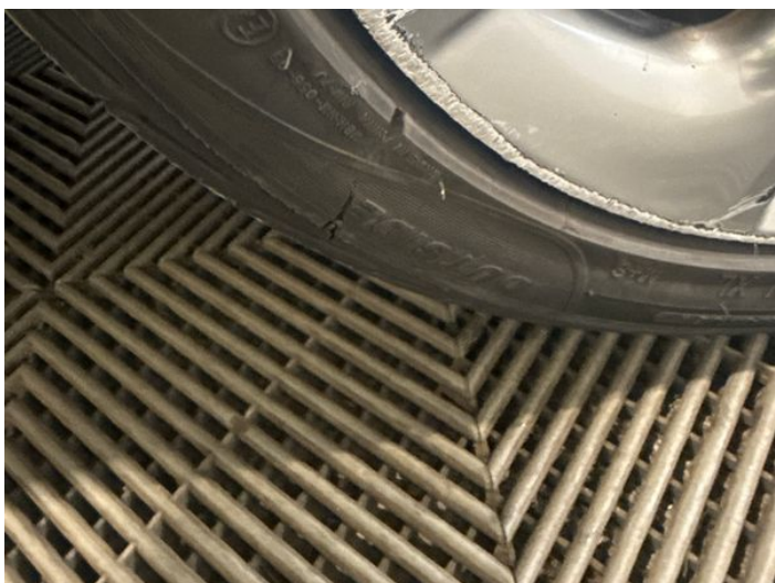
23: Tyre osf Damaged Replace
