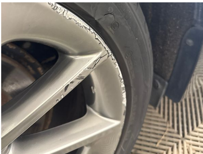
24: Tyre osr Damaged Replace
