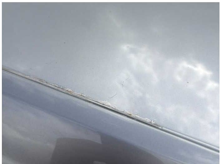
14: Roof Dented With Paint Damage
