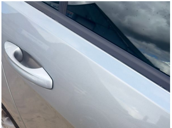
6: Door osr Poor Previous Repair Poor Paint
