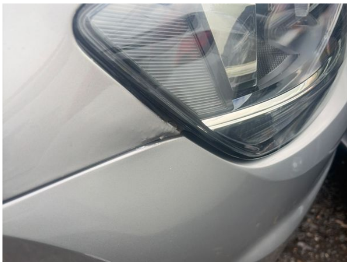
1: Wing osf Dented With Paint Damage
