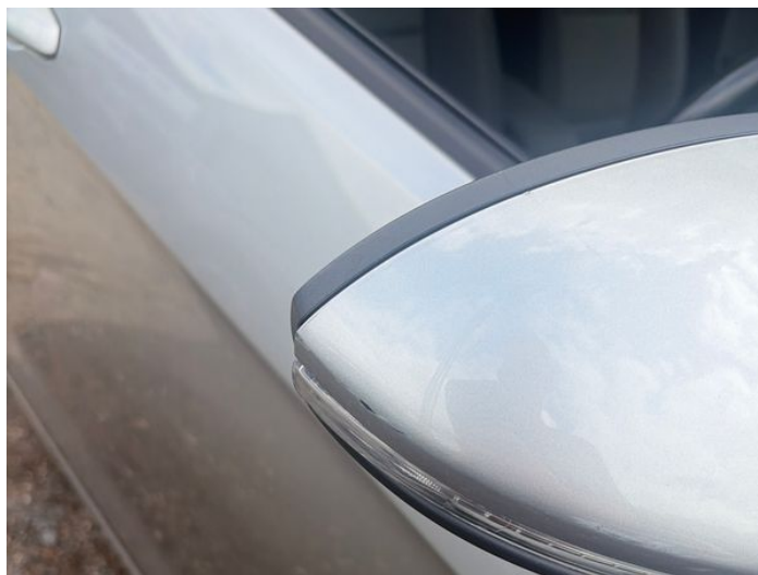
2: Door Mirror Assy osf Scratched (Painted) UpTo 25mm Thru Paint
