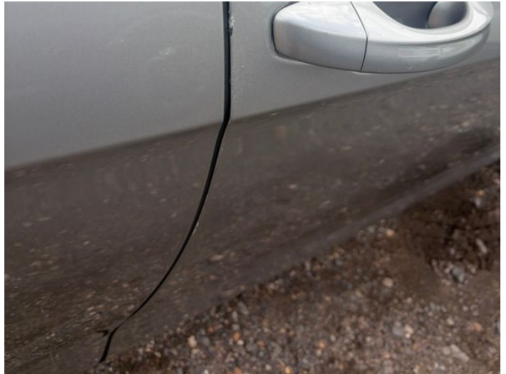
4: Door osf Chipped Edge Chip
