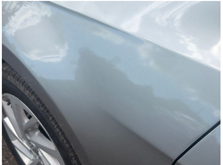
12: Wing nsf Poor Previous Repair Poor Paint
