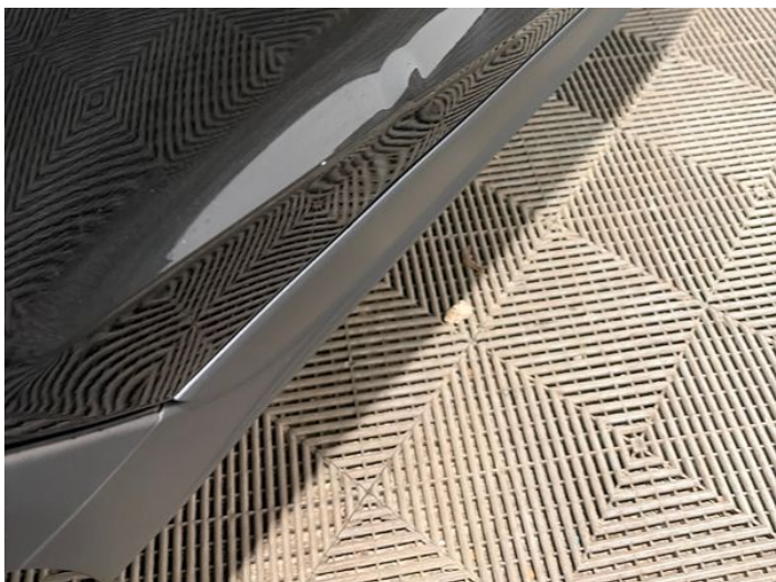
9: Door osr Dented Over 30mm
