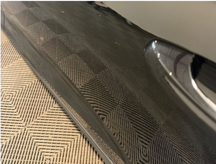
5: Door nsr Chipped 1 To 5
