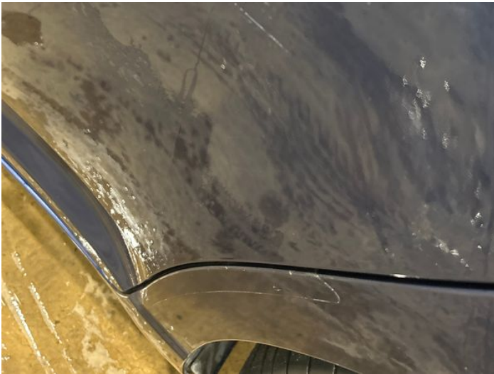
11: Door nsr Scratched UpTo 25mm Thru Paint
