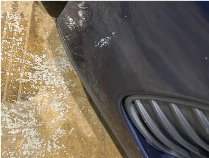
15: Bumper Front Poor Previous Repair Paint Flake
