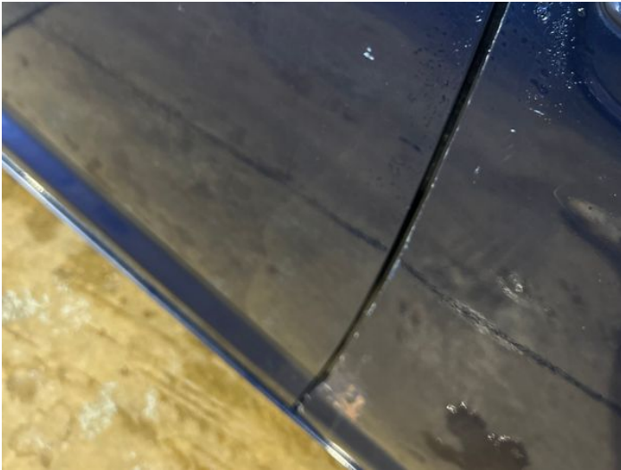
3: Door osr Chipped 1 To 5
