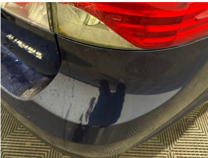
19: Lamp osr Broken Replace
