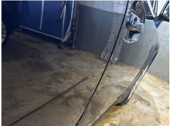
4: Door osr Dented Between 10mm + 30mm
