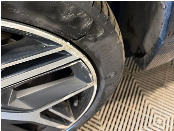
18: Tyre nsf Damaged Replace
