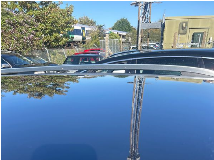
16: Roof Dented 2 Or Less UpTo 10mm
