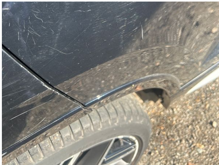
4: Door osr Scratched Over 25mm Thru Paint
