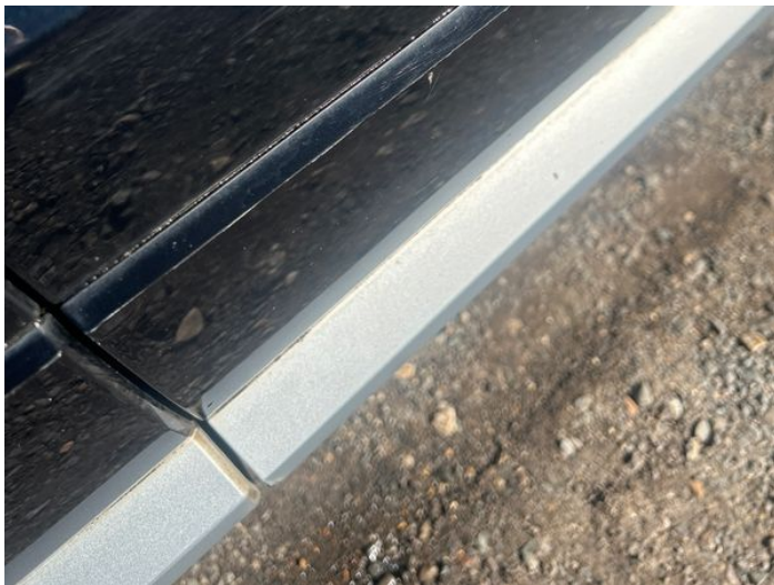
3: Door osf Scratched Over 25mm Thru Paint
