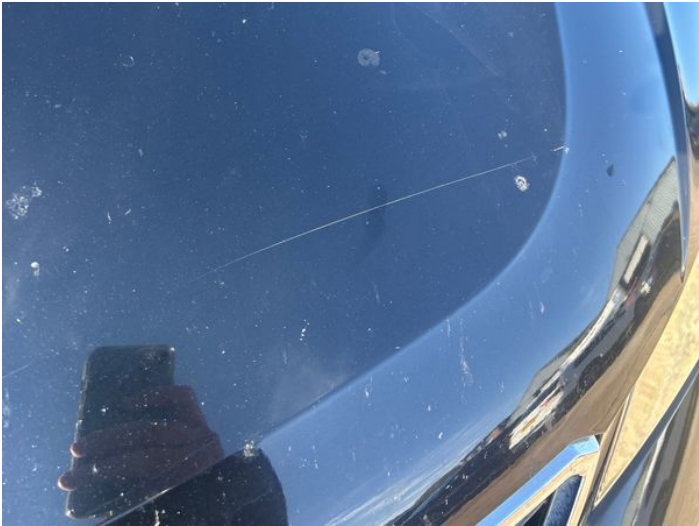
15: Bonnet Scratched Over 25mm Thru Paint
