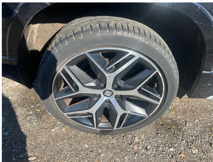
6: Wheel osr Corroded Light
