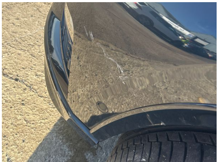
14: Bumper Front Scratched Over 100mm Thru Paint
