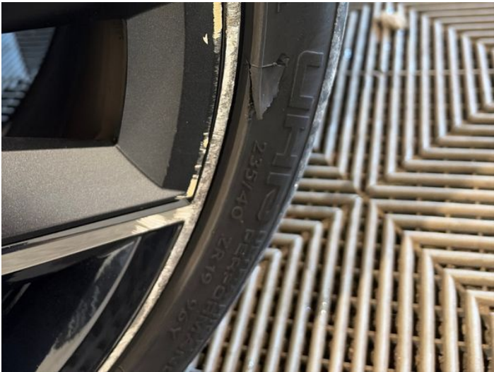
17: Tyre osf Damaged Replace
