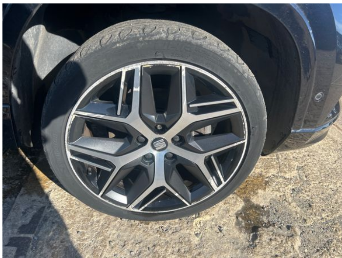
1: Wheel osf Scratched Over 50mm
