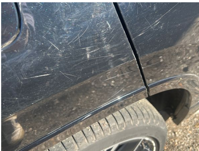
5: Qtr Panel osr Scratched Over 25mm Thru Paint
