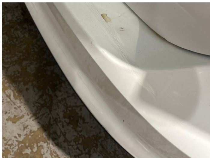
6: Bumper Rear Poor Previous Repair Paint Flake
