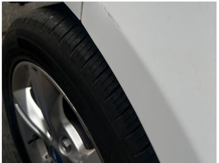
12: Wing nsf Scratched Over 25mm Thru Paint
