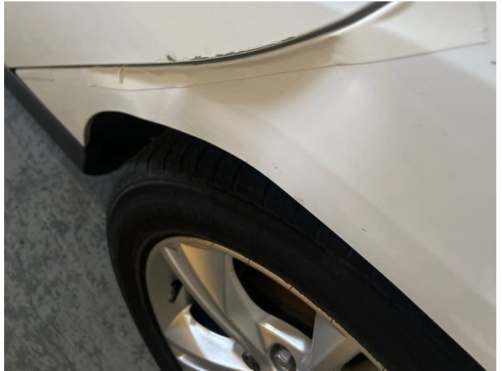
10: Door nsr Scratched Over 25mm Thru Paint
