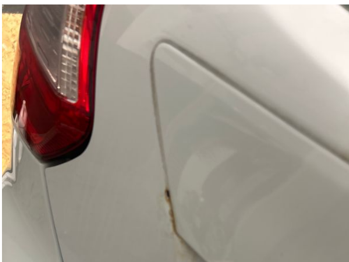
7: Tailgate Rusted Over 5mm
