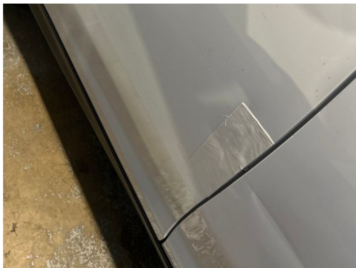
4: Door osr Dented With Paint Damage
