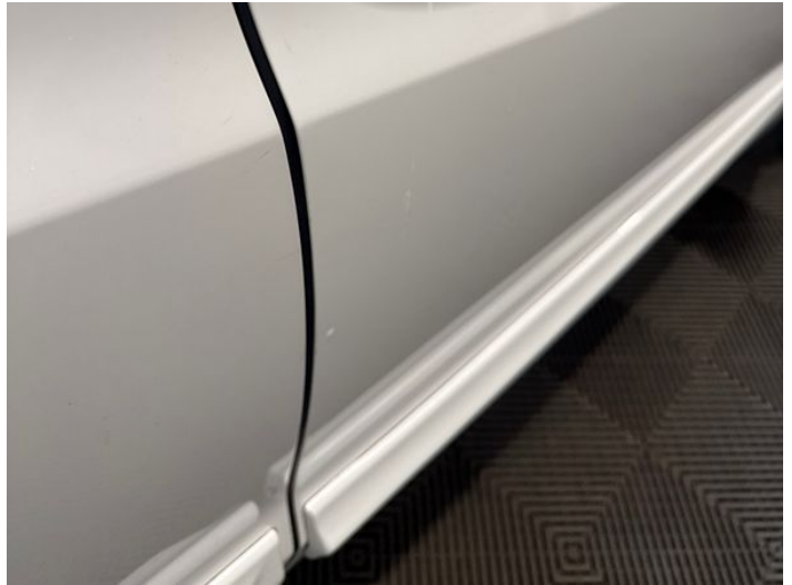
10: Door osf Chipped Edge Chip
