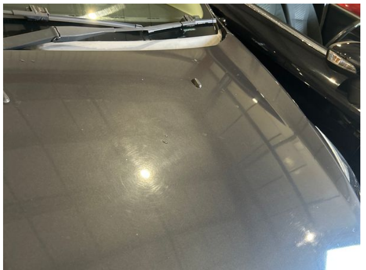
14: Bonnet Poor Previous Repair Poor Paint
