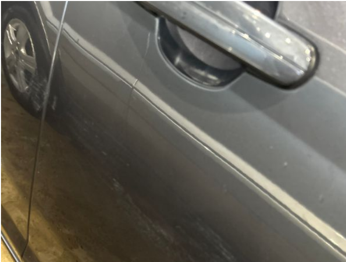
3: Door osf Scratched Over 25mm Thru Paint
