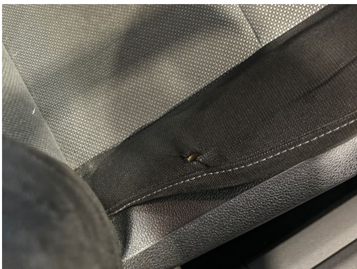
17: Seat Base Cover osf Holed UpTo 3mm
