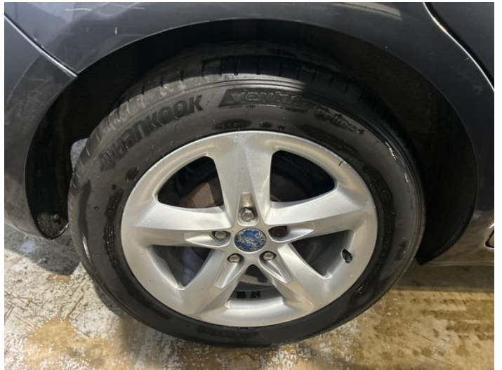
6: Wheel osr Scratched Over 50mm
