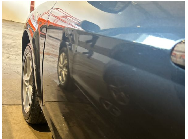
12: Door nsf Poor Previous Repair Poor Paint
