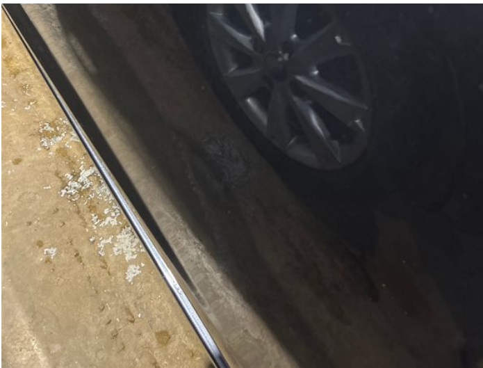
11: Door nsr Chipped 1 To 5
