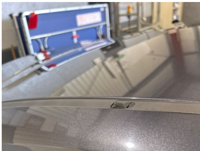
16: C Post os Dented Between 10mm + 30mm
