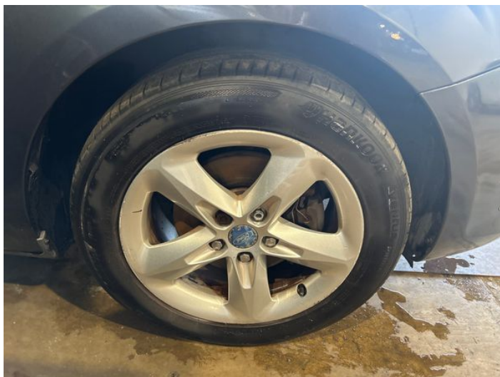
1: Wheel osf Scratched Over 50mm
