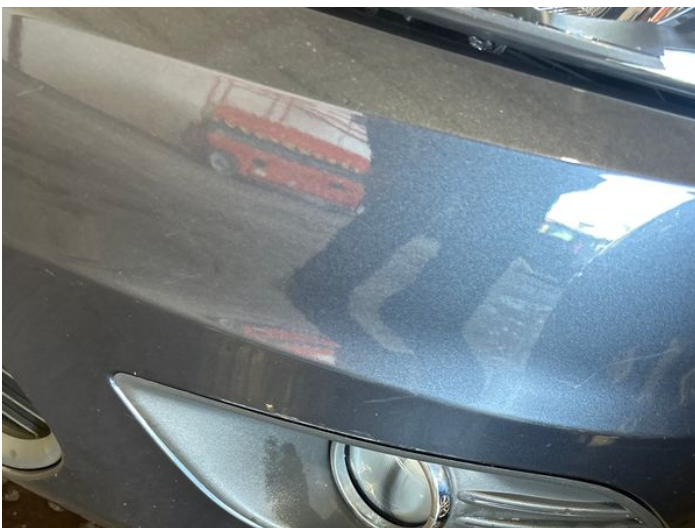
13: Bumper Front Scratched Over 100mm Thru Paint
