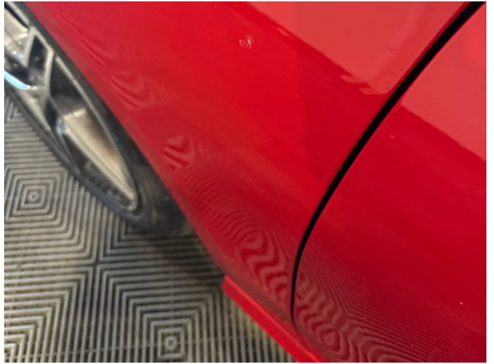
4: Wing nsf Scratched UpTo 25mm Thru Paint
