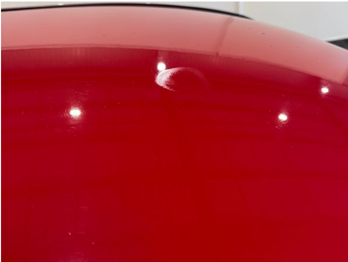
23: Roof Scratched Over 25mm Thru Paint
