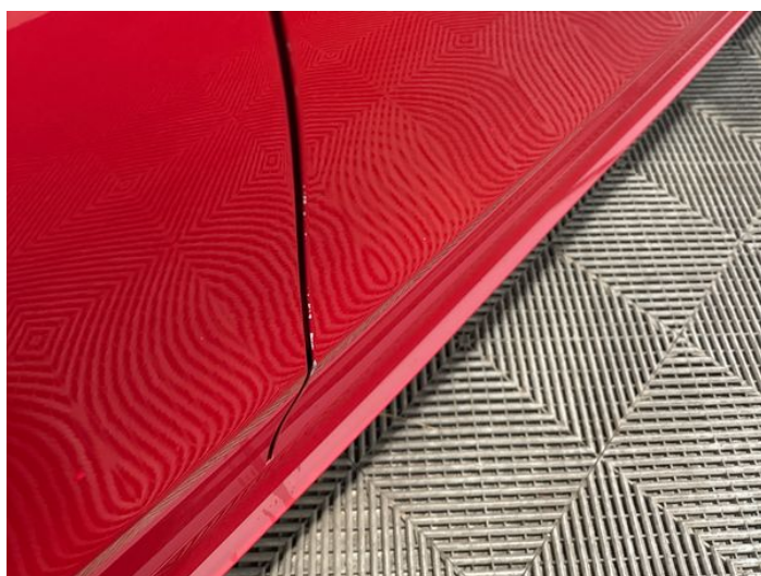
18: Door osf Chipped Edge Chip
