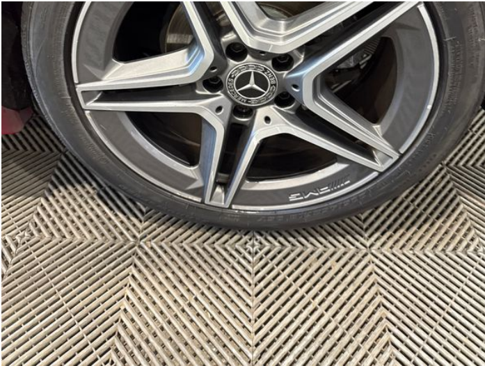
9: Wheel nsr Scratched Over 50mm
