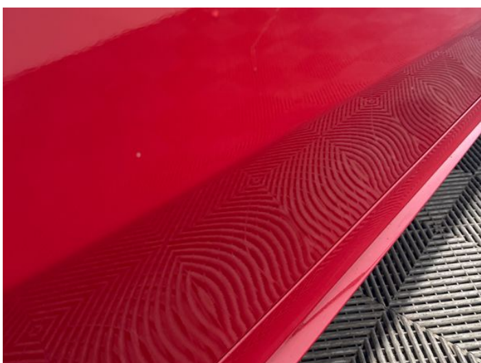
19: Door osf Poor Previous Repair Poor Paint
