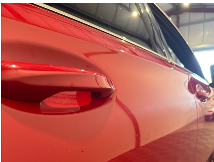
17: Door osr Poor Previous Repair Rippled Up To 30%
