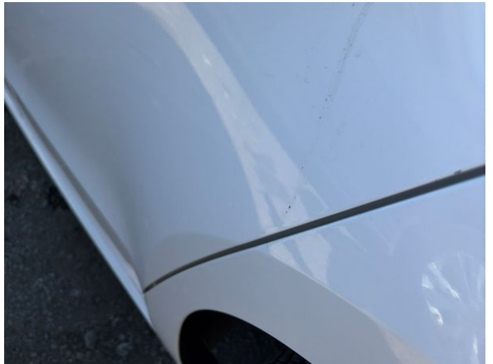
6: Door nsr Scratched Over 25mm Thru Paint
