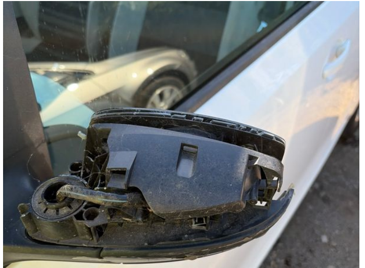
4: Door Mirror Assy nsf Broken Replace
