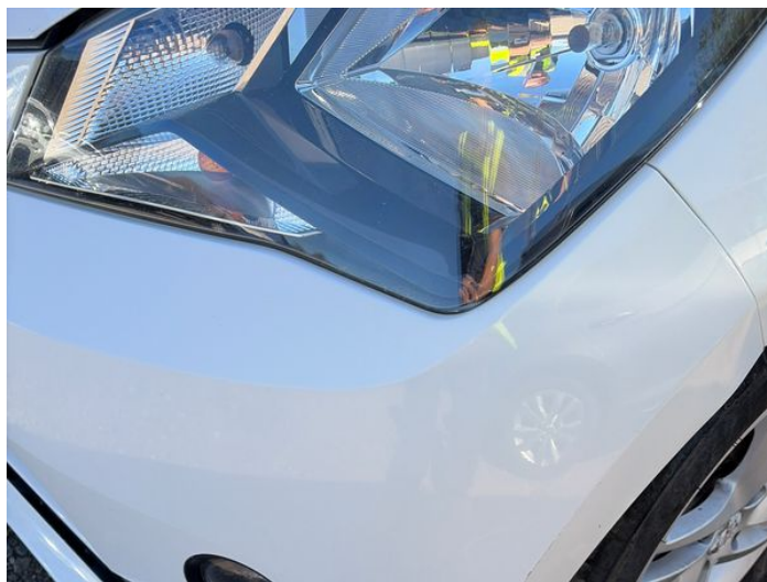
2: Bumper Front Dented With Paint Damage
