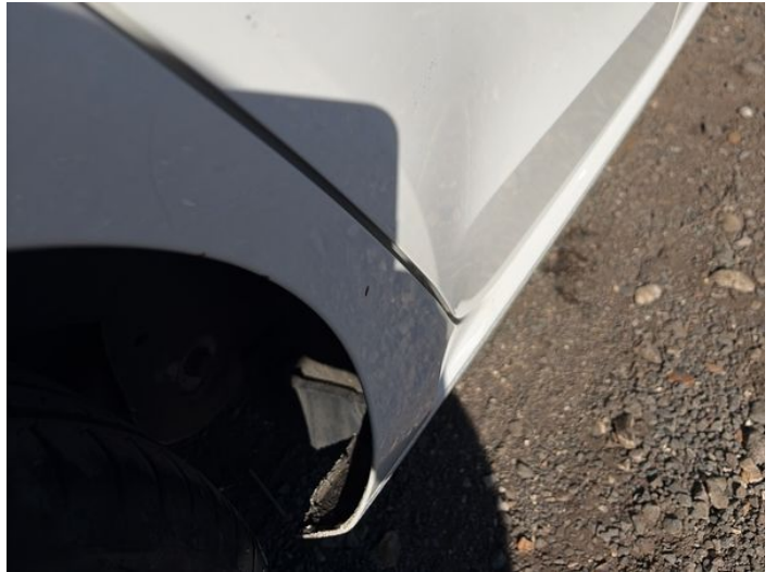
10: Door osf Scratched Over 25mm Thru Paint
