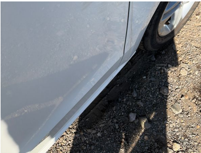
11: Door osf Dented With Paint Damage
