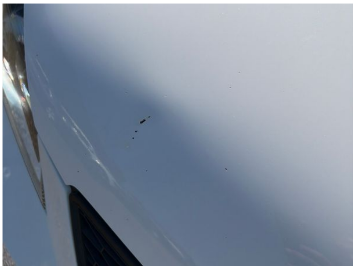
1: Bonnet Dented With Paint Damage
