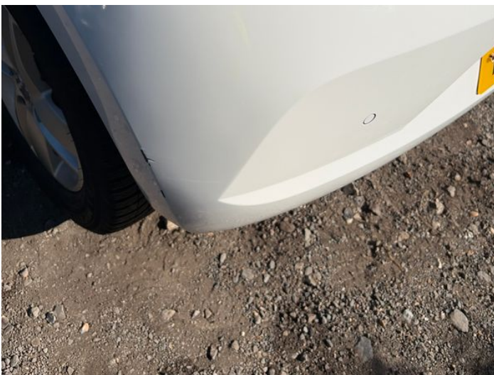
7: Bumper Rear Dented With Paint Damage
