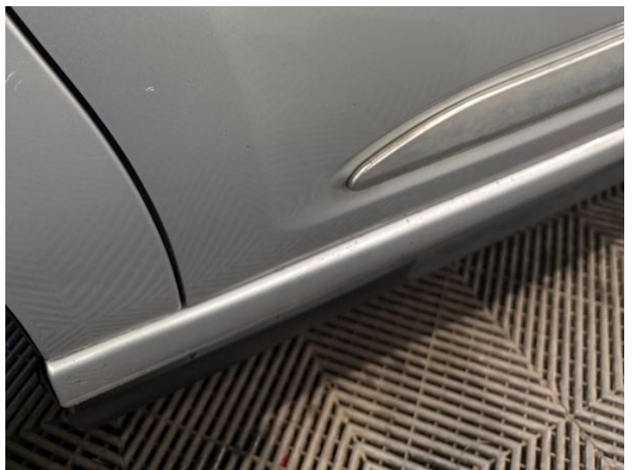
8: Door nsf Chipped 1 To 5
