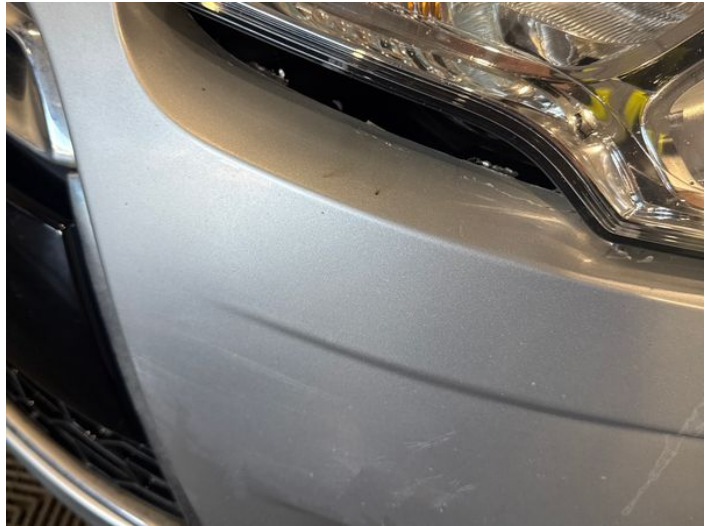
4: Bumper Front Moulding Missing Replace
