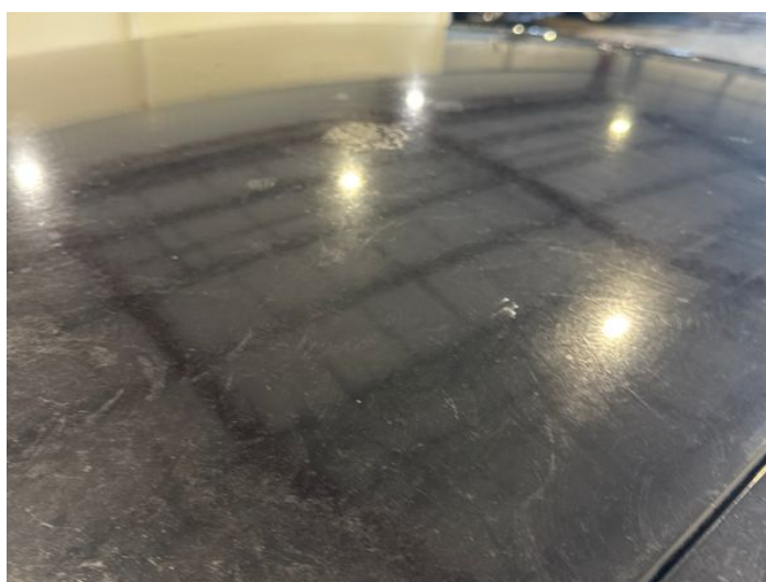
14: Roof Scratched Over 25mm Thru Paint
