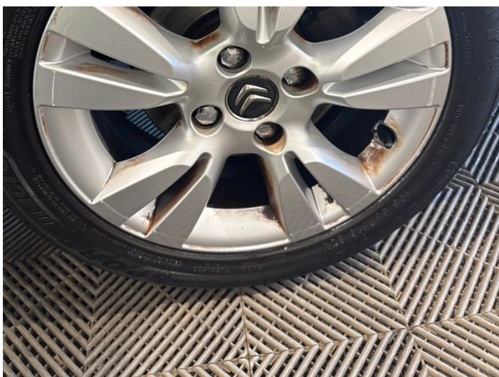
19: Wheel osf Scratched Over 50mm
