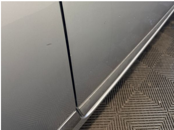
15: Door osf Chipped Edge Chip
