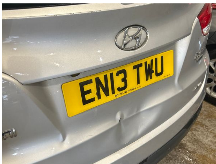
8: Tailgate Dented With Paint Damage
