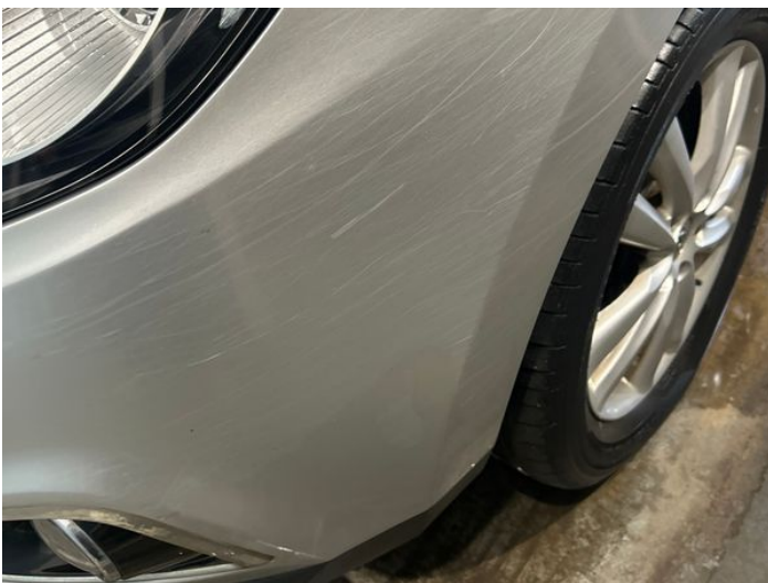
13: Bumper Front Scratched Over 100mm Thru Paint
