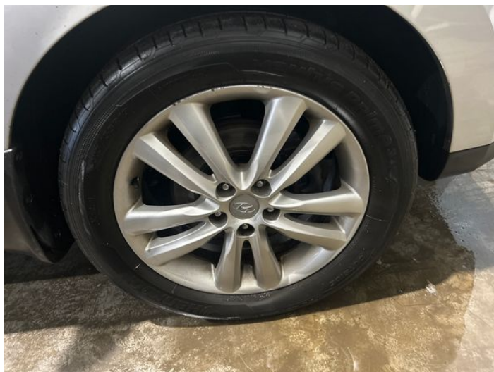
1: Wheel osf Scratched Over 50mm
