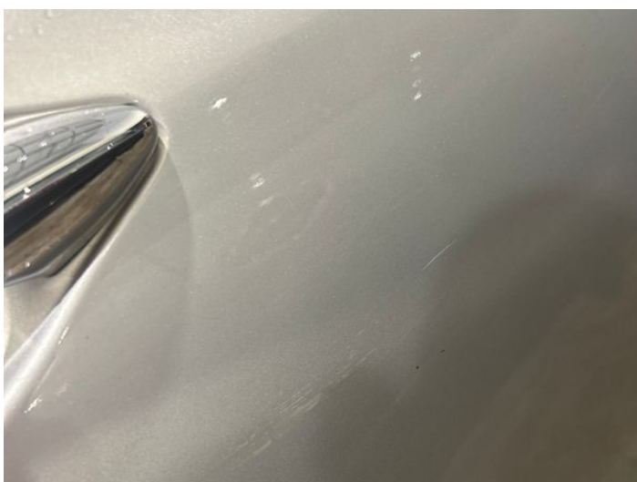
5: Door osr Scratched Over 25mm Thru Paint
