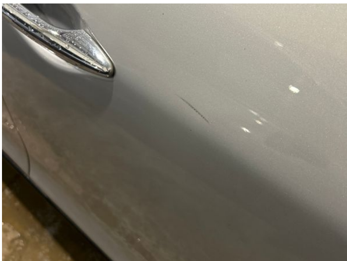
3: Door osf Scratched UpTo 25mm Thru Paint
