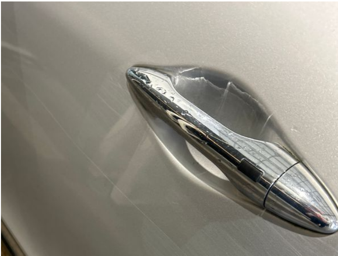
11: Door nsf Scratched Over 25mm Thru Paint
