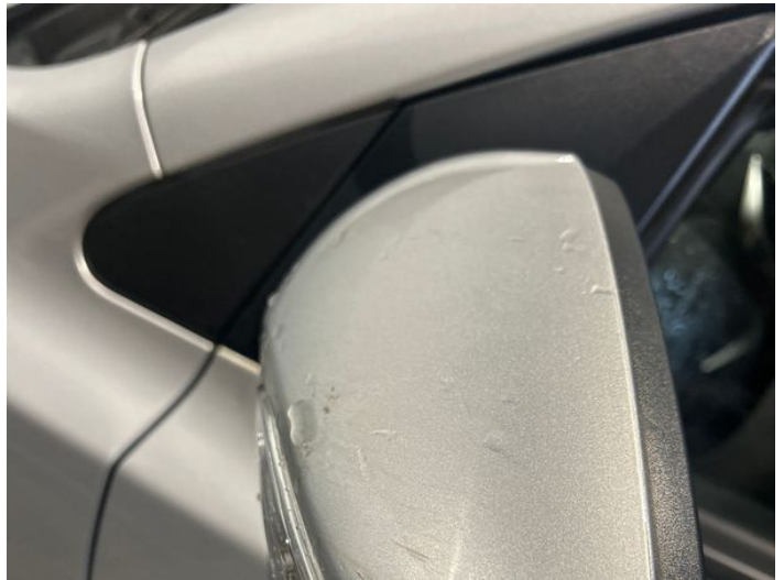
12: Door Mirror Assy nsf Scratched (Painted) UpTo 25mm Thru Paint
