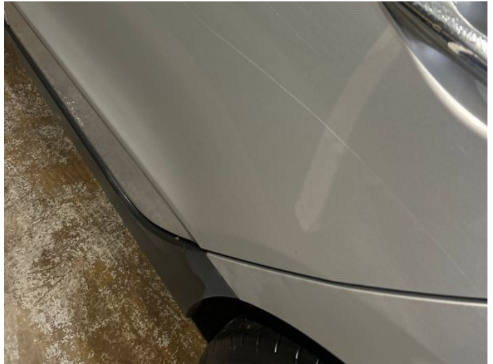
10: Door nsr Scratched Over 25mm Thru Paint
