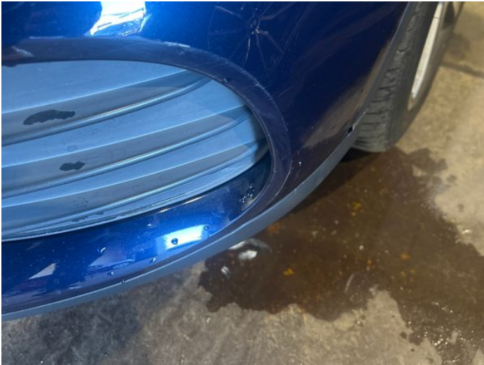
15: Bumper Front Scratched 25 to 100mm Thru Paint
