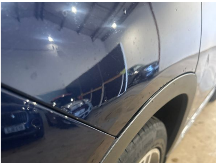
7: Qtr Panel osr Dented Between 10mm + 30mm
