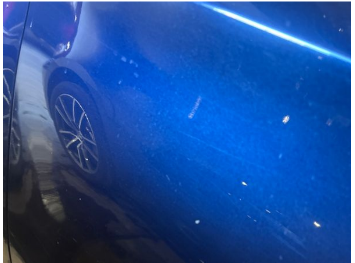
12: Door nsf Chipped 1 To 5
