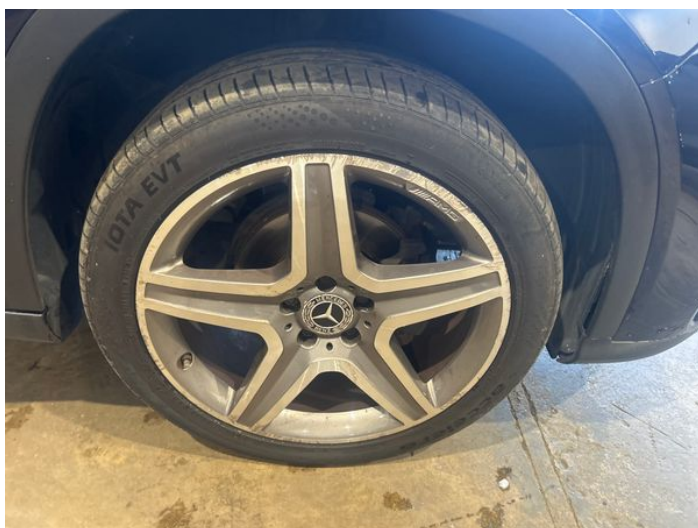
1: Wheel osf Scratched Over 50mm
