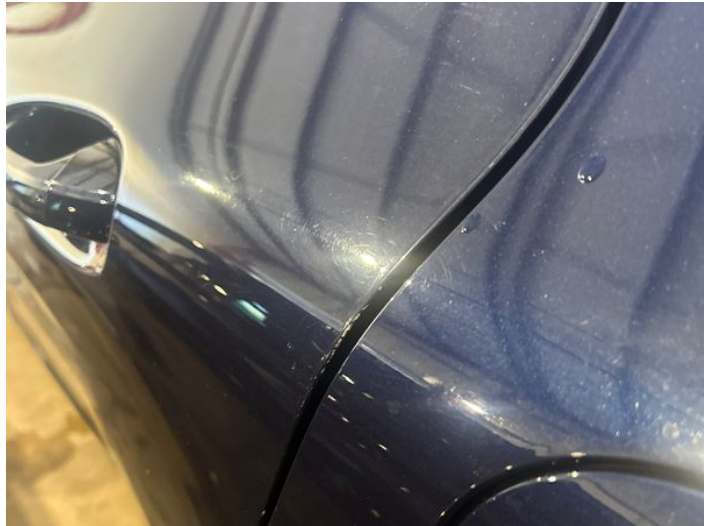
10: Door nsr Chipped Edge Chip
