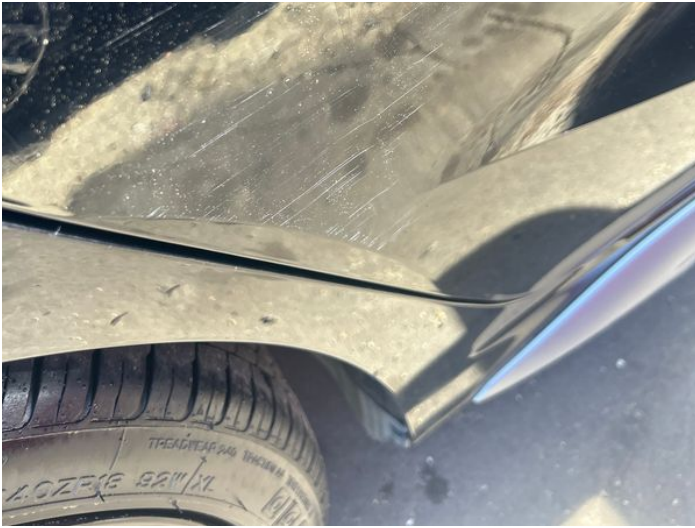
3: Door osr Scratched Over 25mm Thru Paint
