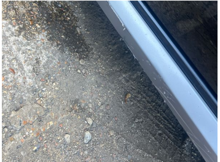
10: Sill Panel Trim ns Scratched (Painted) Over 25mm Thru Paint
