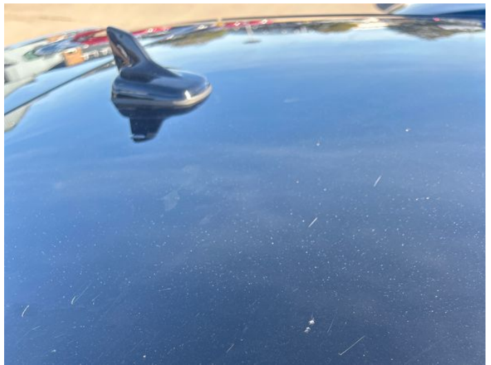
18: Roof Scratched Over 25mm Thru Paint
