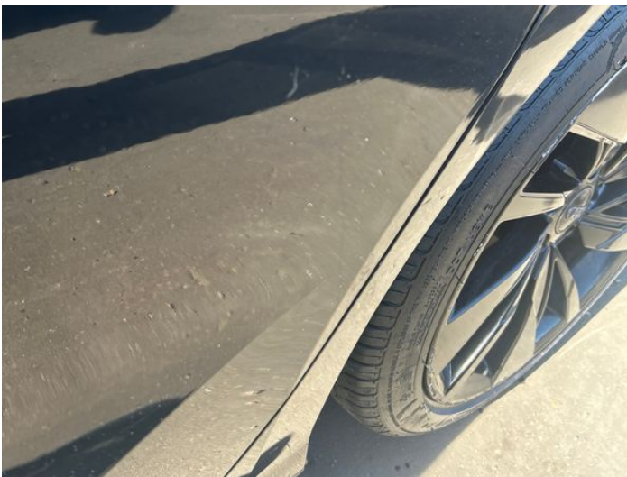
11: Door nsr Scratched UpTo 25mm Thru Paint
