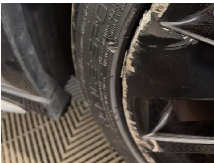
19: Tyre osf Damaged Replace
