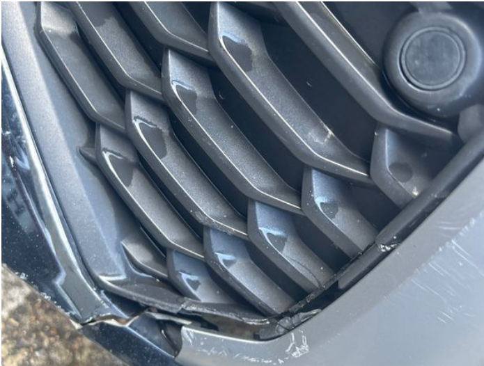
15: Bumper Front Grill Broken Replace
